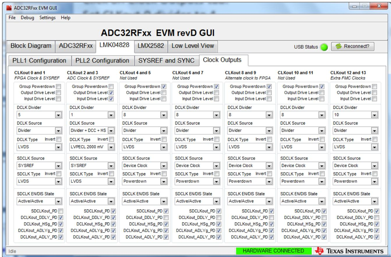
Figure 15. Updated LMK0828 Clock Outputs Tab
