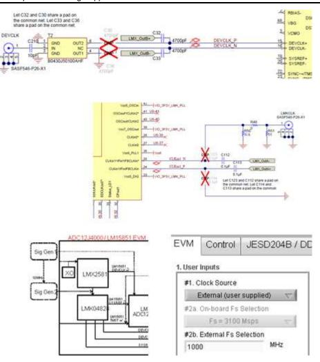
Figure C-1. Configuration for Optional Clocking Support
