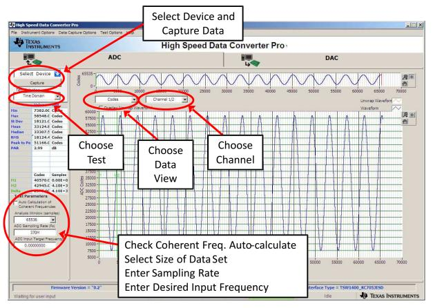
Figure 3-5. High Speed Data Converter Pro (HSDC) GUI
