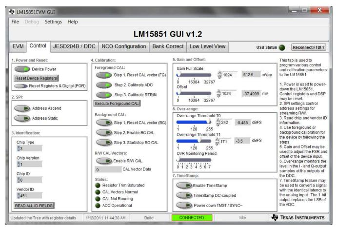
Figure 3-4. Configuration GUI ADC Control
