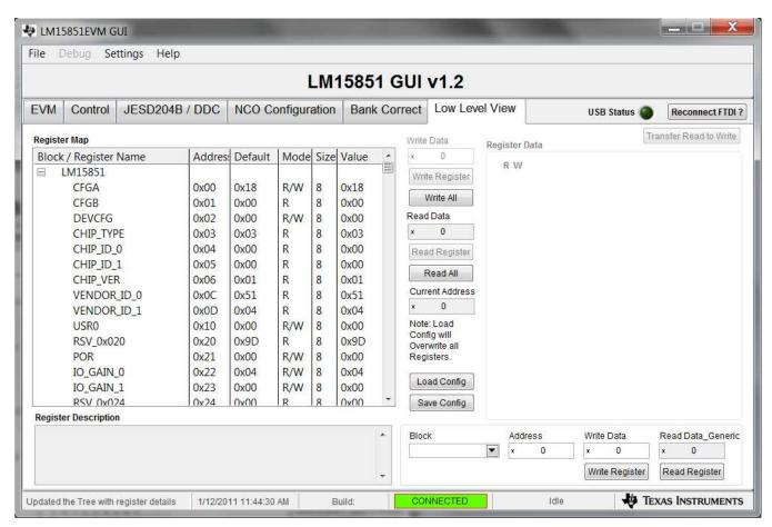
Figure 4-1. Low-Level Register Control Tab
