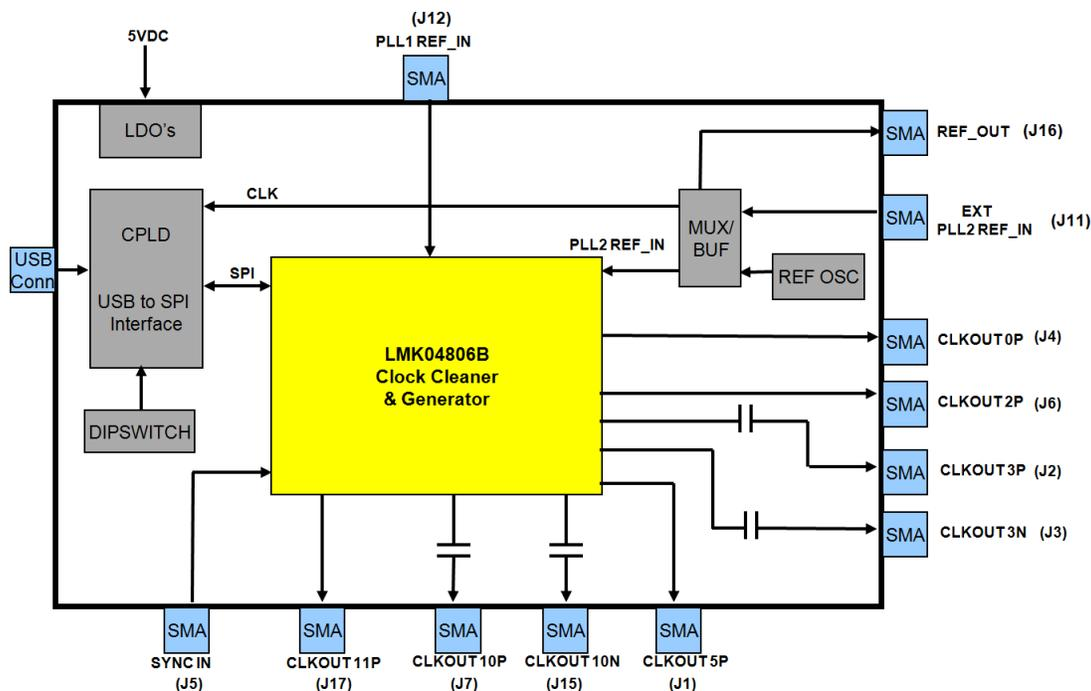
**Figure 1. TSW4806EVM Block Diagram**
