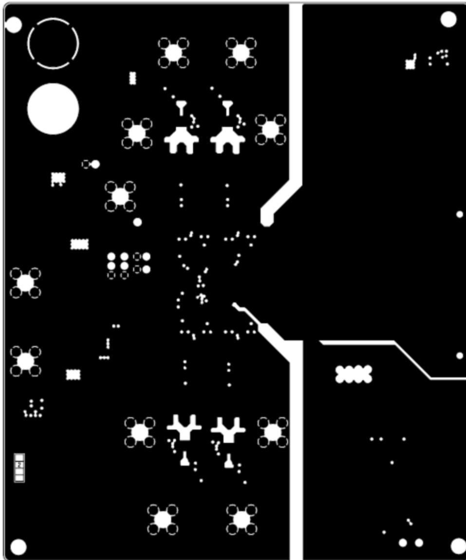
Figure 18. ADS5263EVM Internal Layer 1, Ground – Top View
