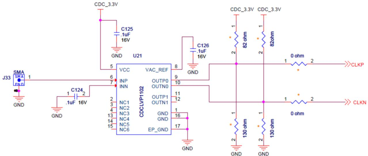
Figure 3. ADS5263 Clocking Using a LVPECL Buffer
