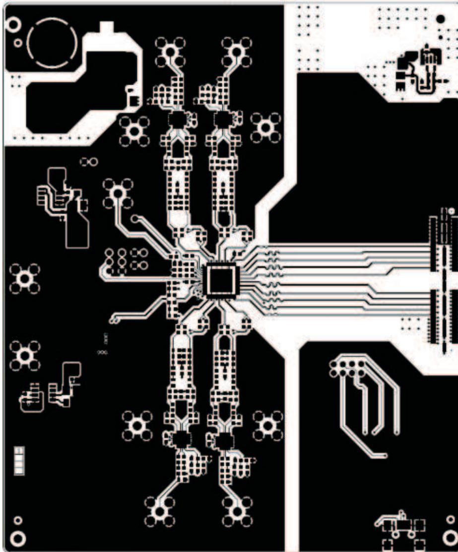
Figure 17. ADS5263EVM Top Layer Copper – Top View
