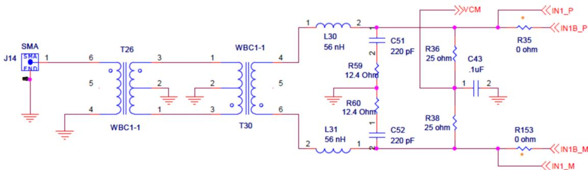
Figure 4. Input Drive Circuit – Using Transformers
