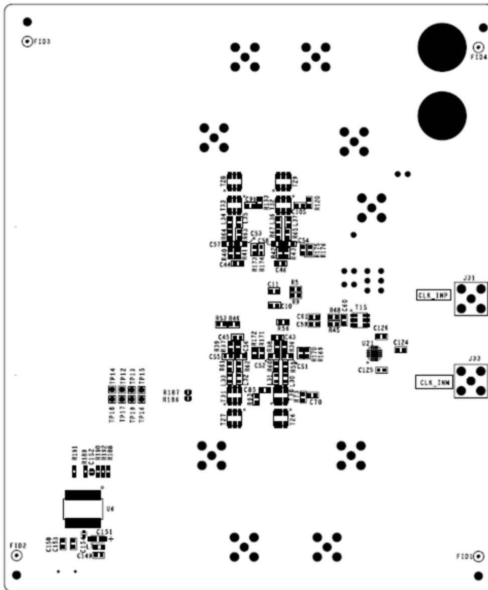
Figure 16. ADS5263EVM Bottom Layer Assembly Drawing – Bottom View
