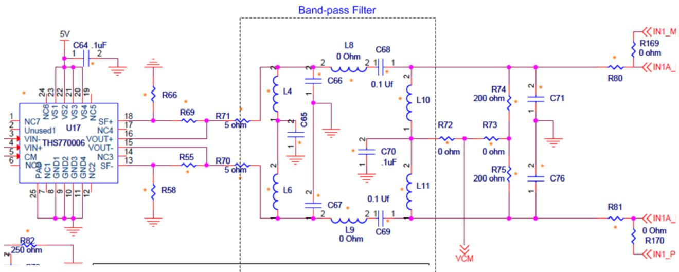
**Figure 6. Band-Pass Filter**
