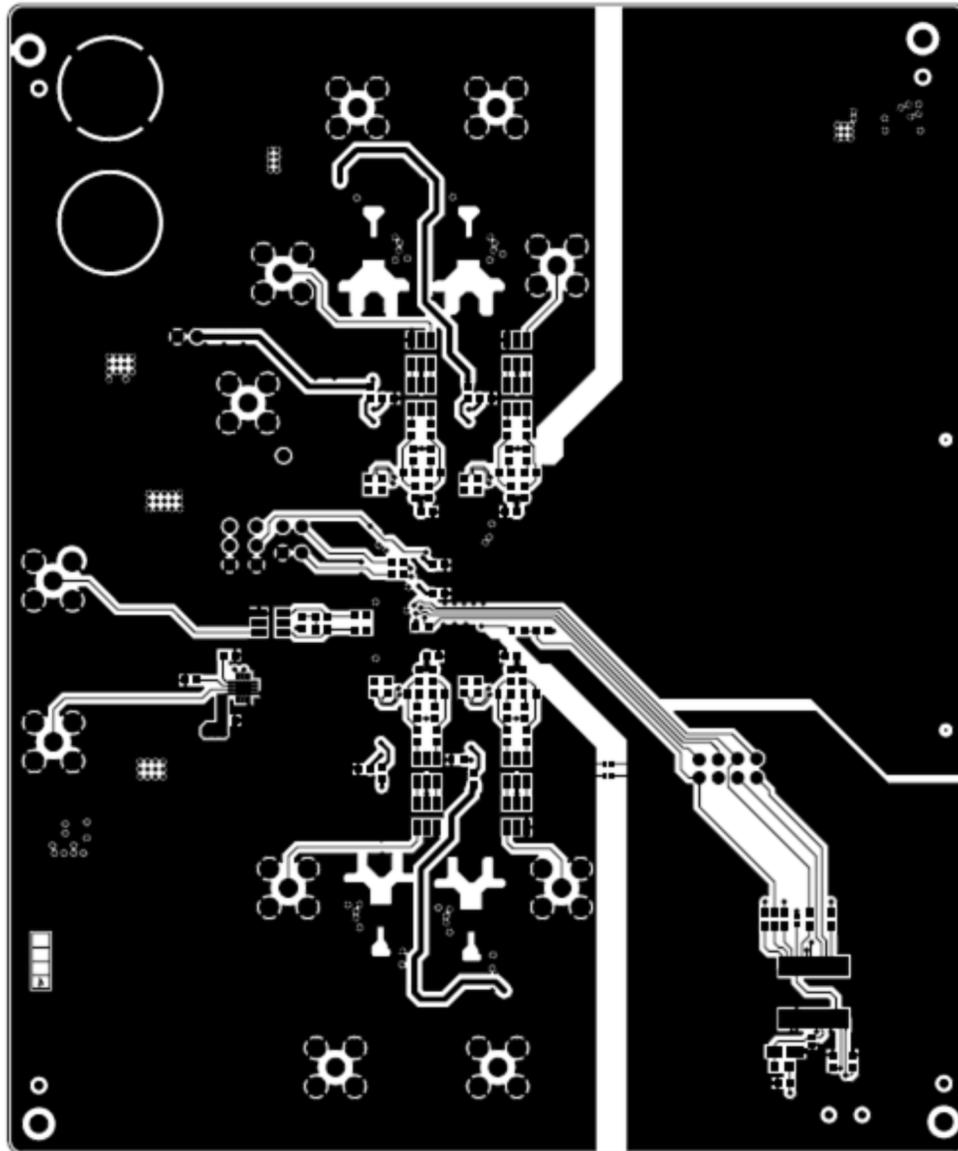
Figure 20. ADS5263EVM Bottom Layer Copper – Top View
