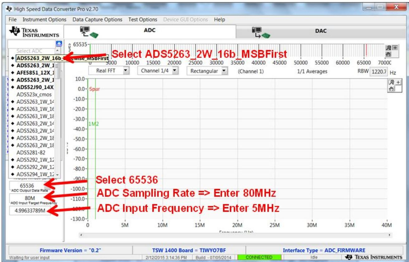
Figure 11. Successful Interface Between TSW Card and Computer
