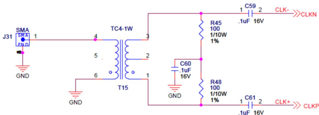
**Figure 2. ADS5263 Sine Wave Clocking Using Transformer**
