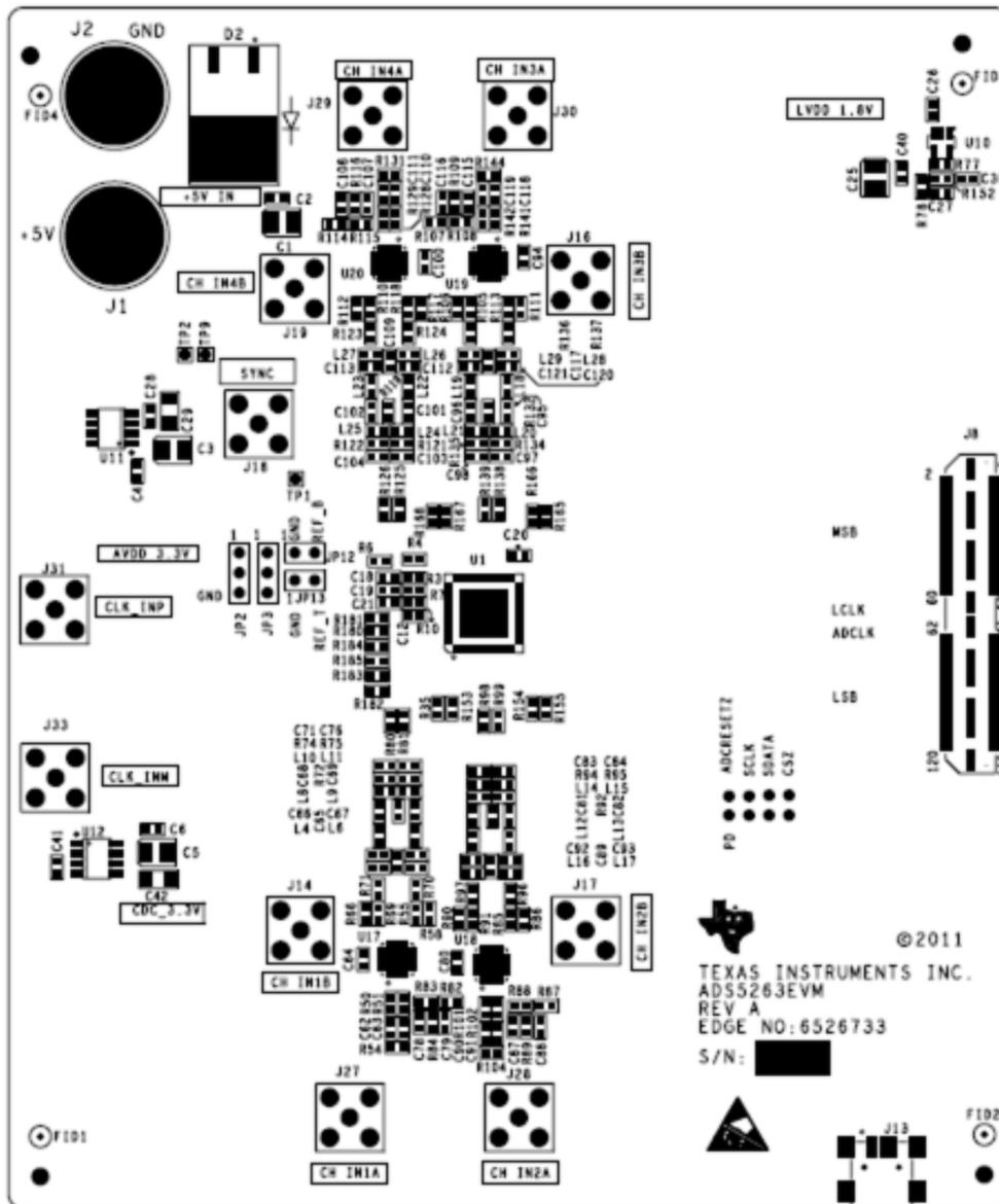
Figure 15. ADS5263EVM Top Layer Assembly Drawing – Top View
