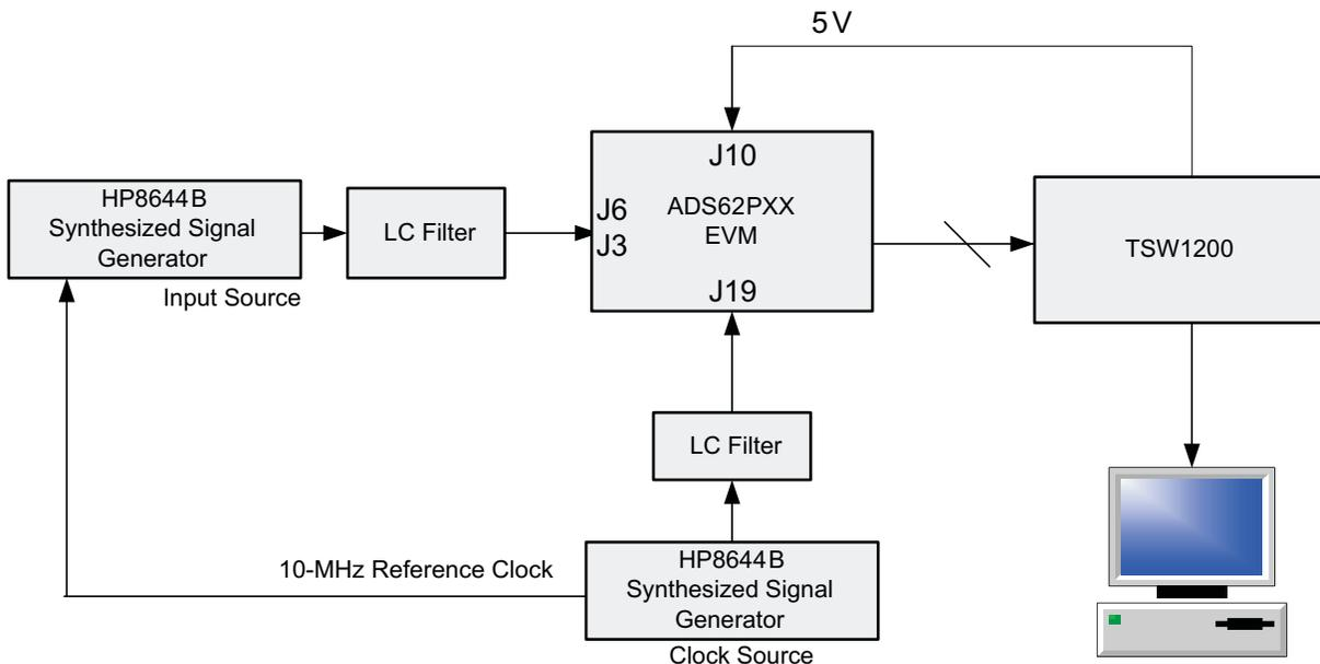
1. The ADS62Pxx evaluation module (EVM) contains a linear power supply solution to provide the necessary voltage rails to the analog-to-digital converter (ADC) and associated circuits. Connect +5V to J10 and GND to J12.
