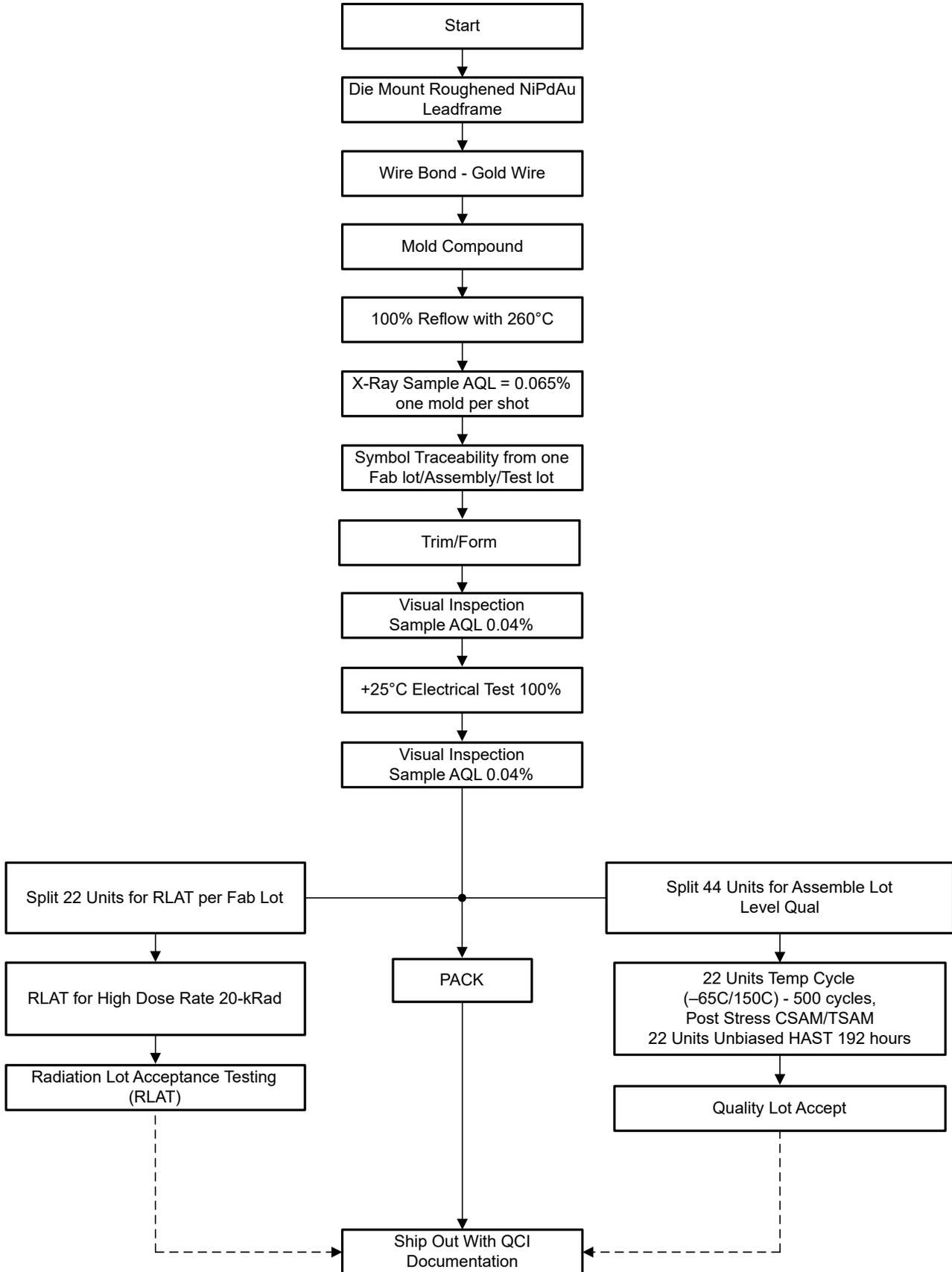
**Figure 2-1. AFE11612-SEP Space-Enhanced Plastic Production Flow Chart**
