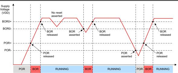
Figure 3-2. POR and BOR vs. Supply Voltage (VDD)
