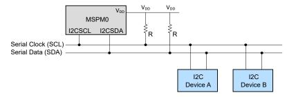
Figure 7-7. Typical I2C Bus Connection
