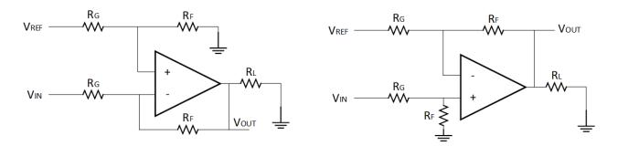
Figure 6-10. GPAMP Circuit in Amplify Mode
