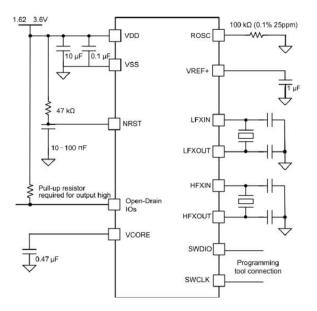
Figure 1-1. MSPM0G Typical Application Schematic
