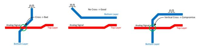
Figure 9-4. Poor and Correct Cross Traces for Analog and High-Frequency Signals
