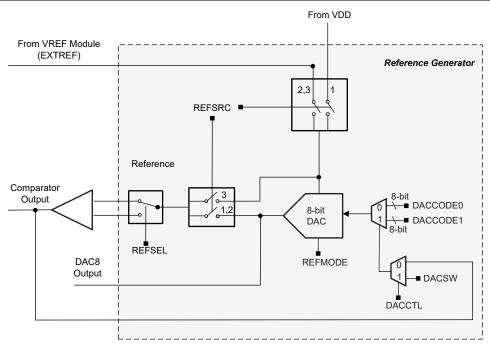
Figure 6-4. 8-Bit DAC Block Diagram
