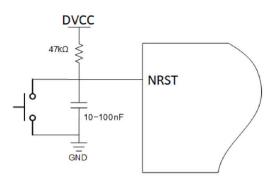
Figure 3-1. NRST Recommended Circuit
