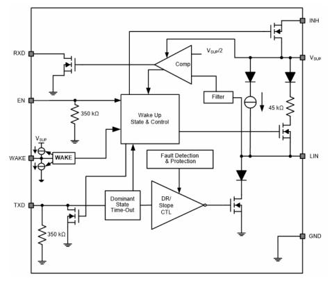
Figure 7-1. Typical LIN TLIN1021A Transceiver
