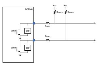
Figure 8-1. Suggested ODIO Circuit
