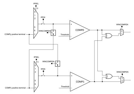
Figure 6-8. Window Comparator Mode
