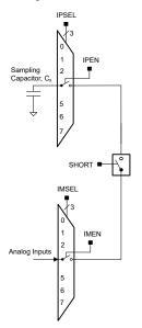
Figure 6-9. Comparator Short Switch
