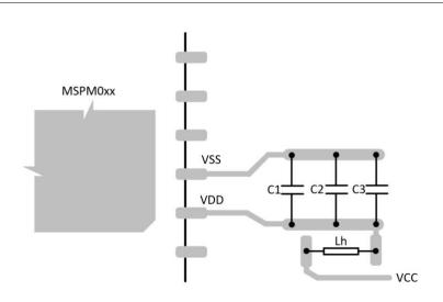
Figure 9-1. Suggested Power Supply Layout
