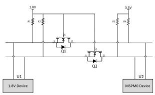
Figure 8-2. Suggested Communication Circuit With 1.8V Device
