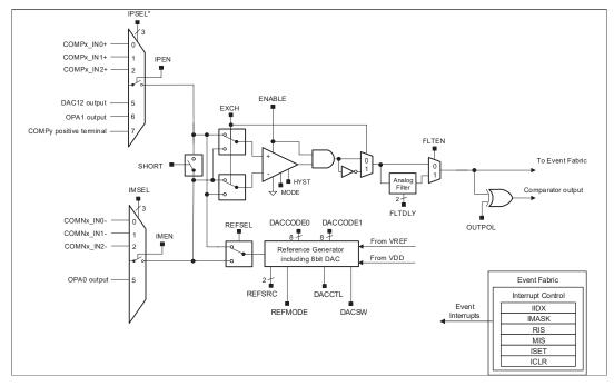
Figure 6-7. Comparator Diagram
