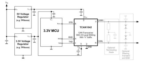
Figure 7-5. Typical CAN Bus Application With MSPM0G
