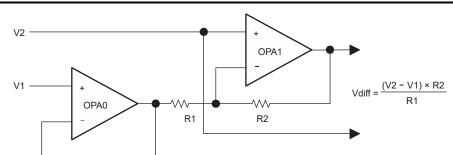
Figure 6-2. Two OPA Differential Amplifier Block Diagram and Equation
