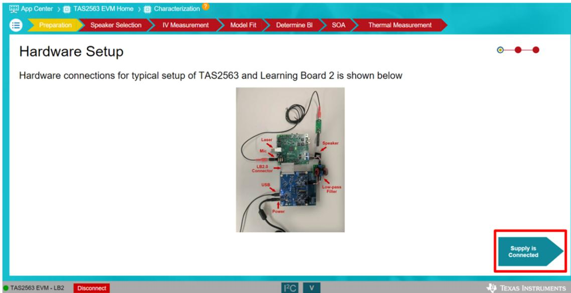
Figure 1-5. Hardware Setup
