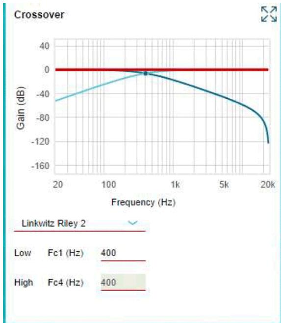
**Figure 2-23. DRC Crossover Filter Controls**
