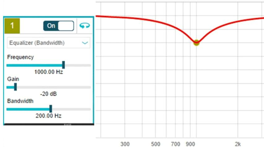
Figure 2-15. Equalizer and Biquad Control
