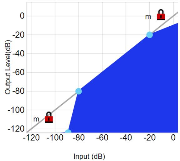
Figure 2-26. Manual Noise Gate Setting
