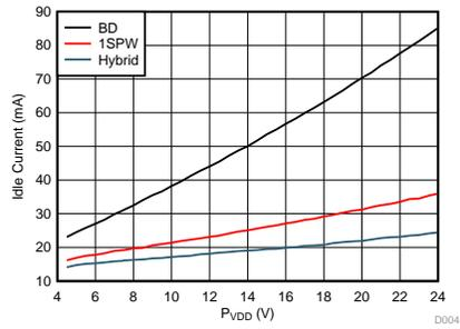
Figure 9. Idle Current vs PVDD on TAS5805M ( $F_{sw} = 384$  kHz,  $10 \mu\text{H} + 0.68 \mu\text{F}$  LC Filter)
