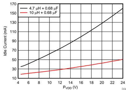
Figure 5. Idle Current vs PVDD on TAS5805M (F<sub>SW</sub> = 768 kHz, BD Mode)
