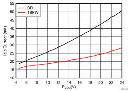
Figure 11. Idle Current vs PVDD on TAS5805M ( $F_{sw} = 768$  kHz,  $10 \mu\text{H} + 0.68 \mu\text{F}$  LC Filter)
