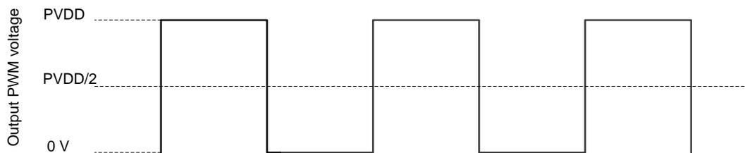
Figure 2. PWM Voltage Waveform
