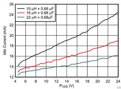
Figure 4. Idle Current vs PVDD on TAS5805M (F<sub>SW</sub> = 384 kHz, Hybrid Mode)
