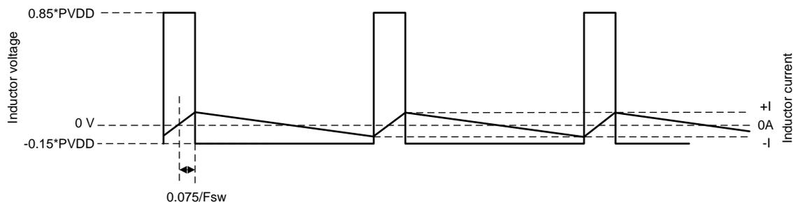
Figure 8. Inductor Voltage and Current (15% Duty-Cycle)
