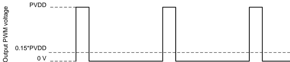
Figure 7. PWM Voltage Waveform (15% Duty-Cycle)
