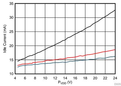
Figure 10. Idle Current vs PVDD on TAS5805M ( $F_{sw} = 384$  kHz,  $22 \mu\text{H} + 0.68 \mu\text{F}$  LC Filter)
