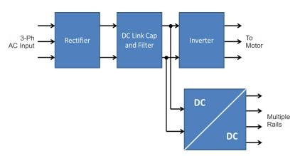
Figure 6. Generation of Multiple Rails in Typical Industrial Drive
