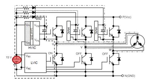
Figure 4. IPM Requiring Single +15 V Supply
