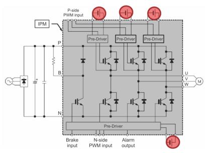
Figure 5. IPM Requiring Individual Power Supplies
