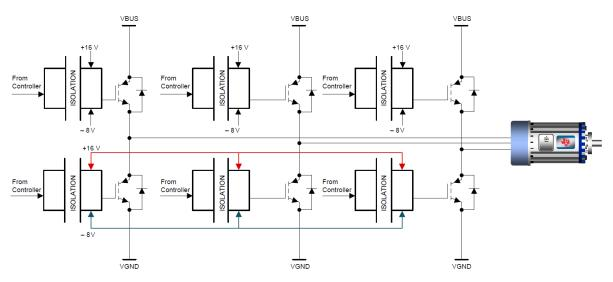
A Lower gate-drivers are powered with a common power supply.
