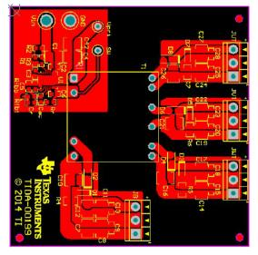
Figure 10. Basic Isolated Board With Single Transformer (Size: 62mm x 55mm)
