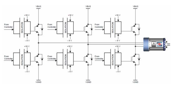
A All gate-drivers are powered with individual isolated power supplies.
