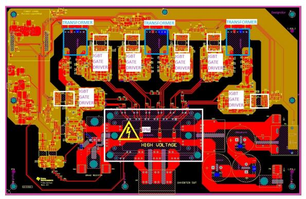
Figure 12. Six IGBT Drivers Driving Single Power Module
