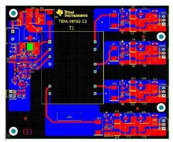
Figure 11. Reinforced Isolated Board With Single Transformer (Size 110mm x 90mm)
