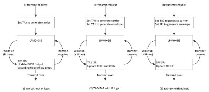
Figure 25. Software Flow for Transmitting One Data Frame With Different Methods
