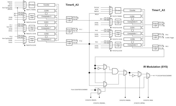
Figure 7. IR Modulation Logic
