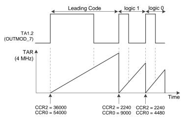
Figure 16. Pulse Distance Protocol, TA1 in Envelope Generation
