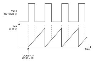
Figure 24. RC5 Protocol, TA0 in Carrier Generation
