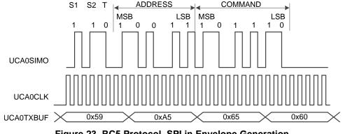
Figure 23. RC5 Protocol, SPI in Envelope Generation
