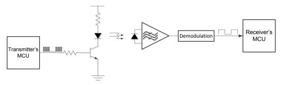
Figure 1. Infrared Modulation and Demodulation
