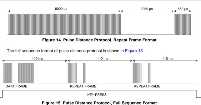
The envelope waveform depends on the frame format. It is easy to quantize all above items with minimum time slot of 0.56 ms (see Table 1).
