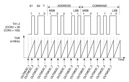
Figure 22. RC5 Protocol, TA1 in Envelope Generation
