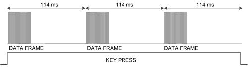
Figure 21. RC5 Protocol, Full Sequence Format
