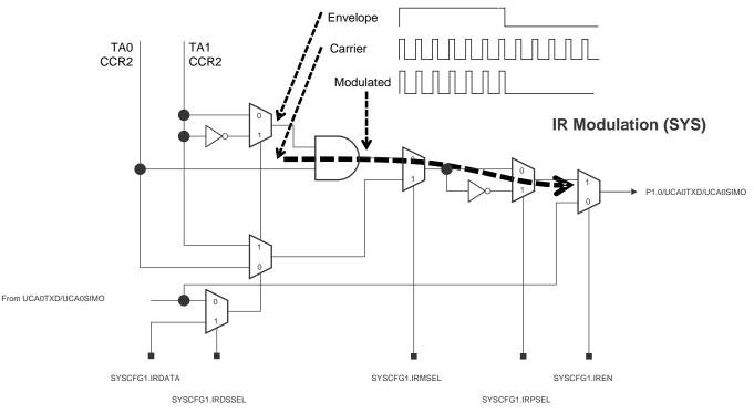
Figure 8. Data Flow in ASK Modulation
