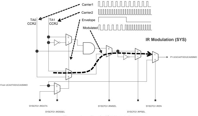
Figure 9. Data Flow in FSK Modulation
