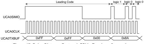
Figure 17. Pulse Distance Protocol, SPI in Envelope Generation
