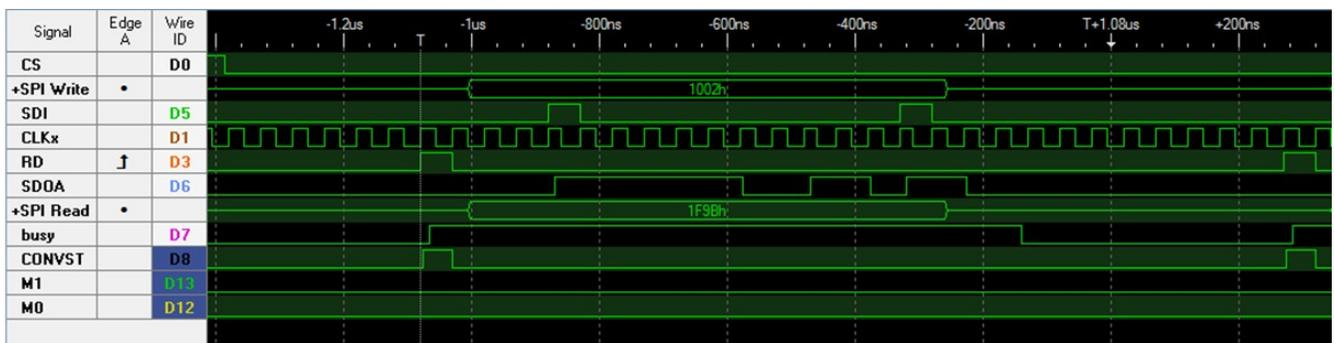
Figure 3. Expanded Mode II Waveform
