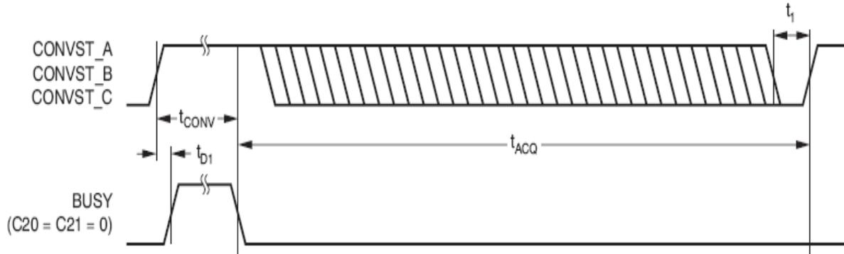
**Figure 3. ADS8556's Acquisition time and Conversion time**
