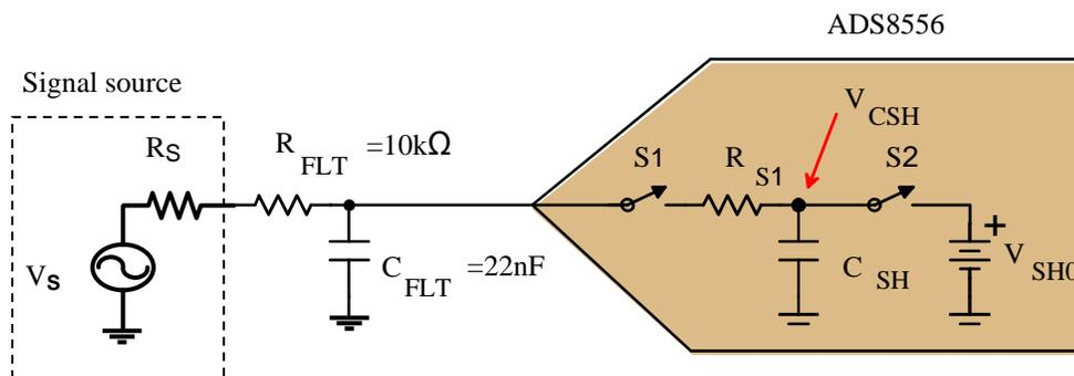
**Figure 2. ADS8556's Driver Circuit Without Front-end Amplifier**
