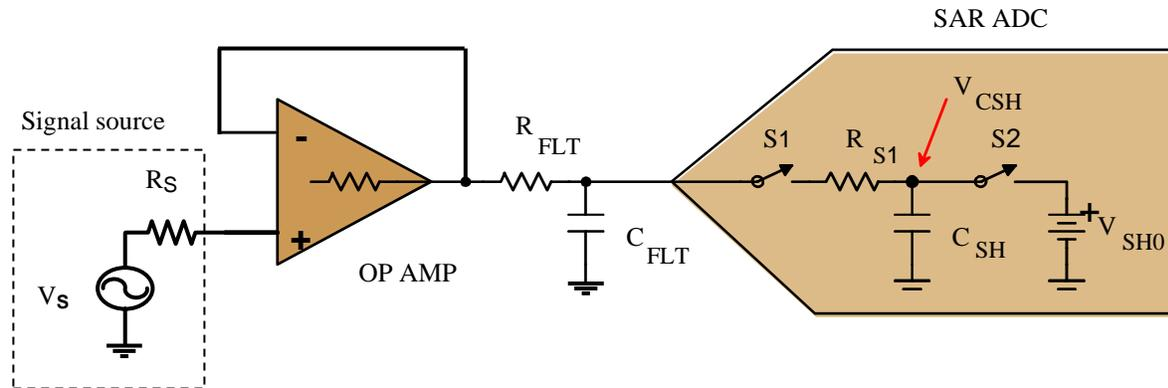
**Figure 1. Typical Driver Circuit for SAR ADC**
