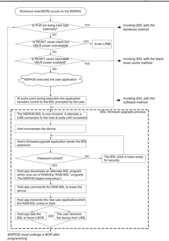
Figure 2. System-Level Description of MSP430 USB Firmware Updates
