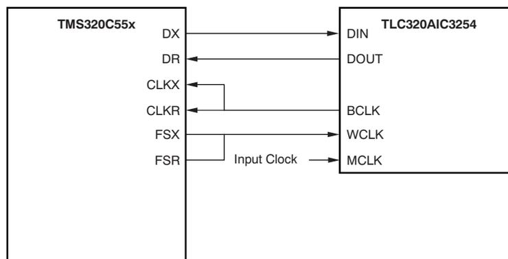
**Figure 1. McBSP Connection to TLV320AIC3254 Codec**
