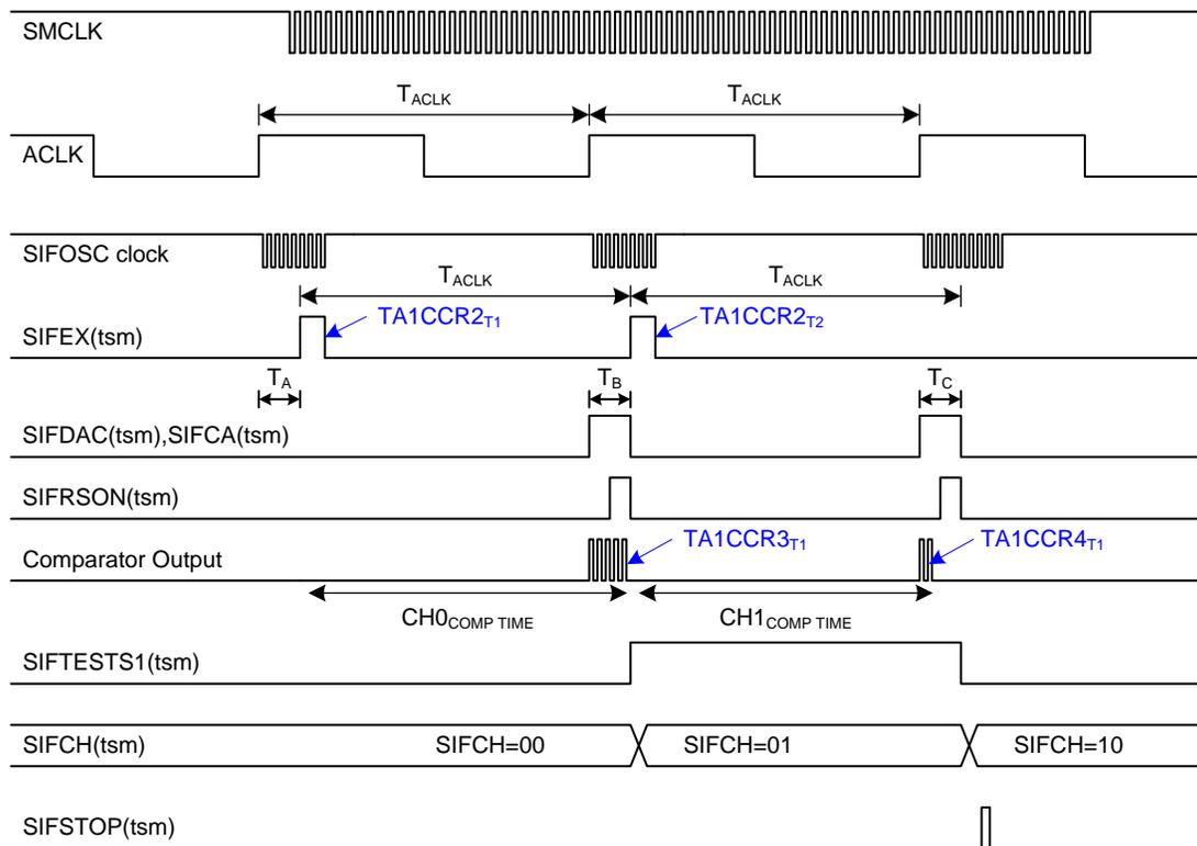
**Figure 5. DCM Operation Example**
