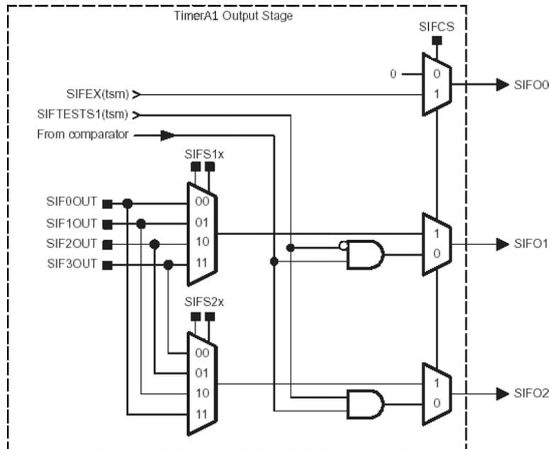
Figure 4. Timer1\_A Output Stage From Scan Interface
