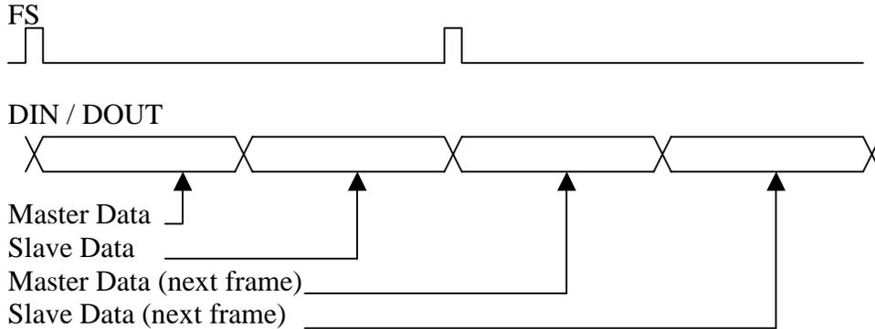
**Figure 4. Master / Slave Communication in Continuous Mode**
