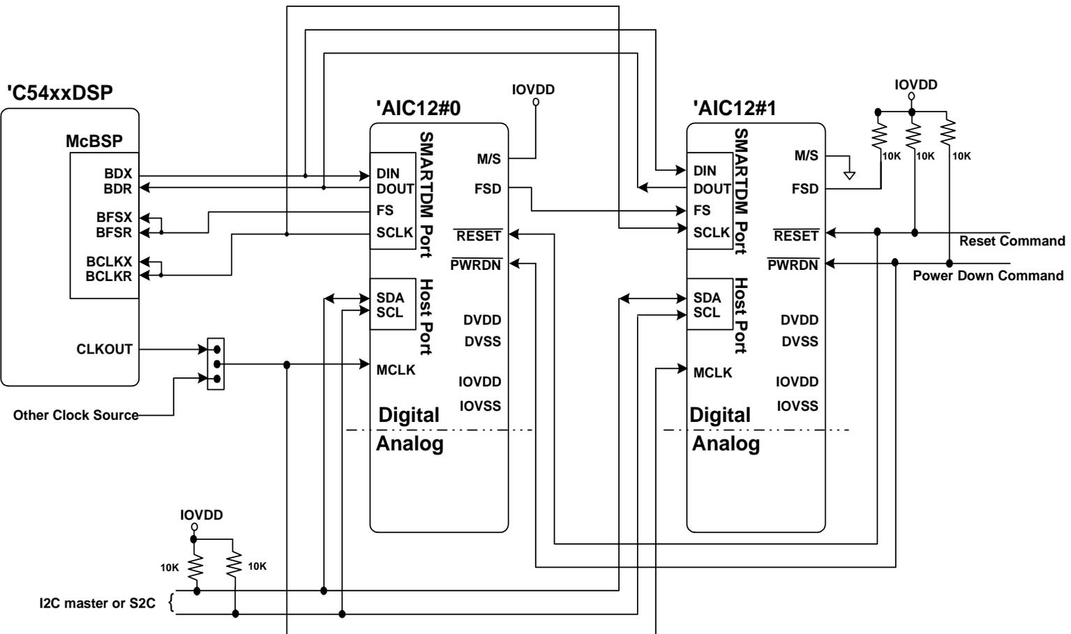
Figure 2. Typical AIC12/C54xx™ DSP Digital Interface, Two-AIC12 Cascade Mode
