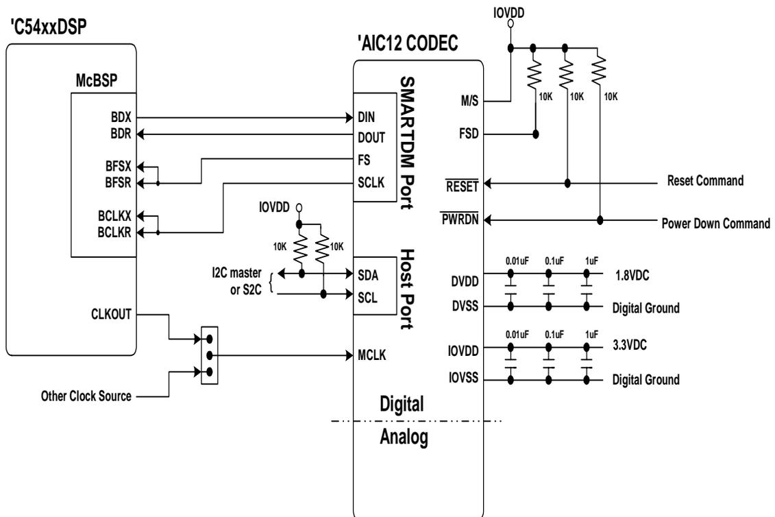
Figure 1. Typical AIC12/C54xx™ DSP Digital Interface, Stand-Alone Master Operation
