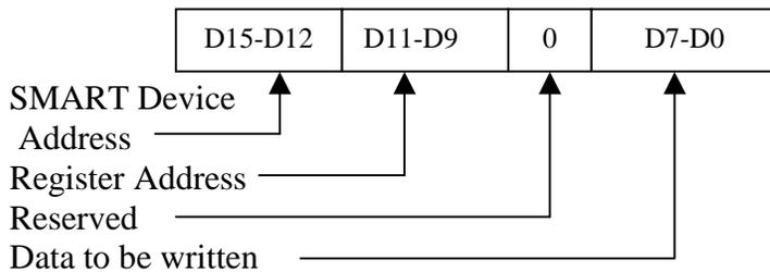
**Figure 6. Control Frame Data Format**
