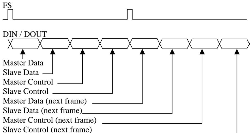
**Figure 3. Master / Slave Communication in Programming Mode**
