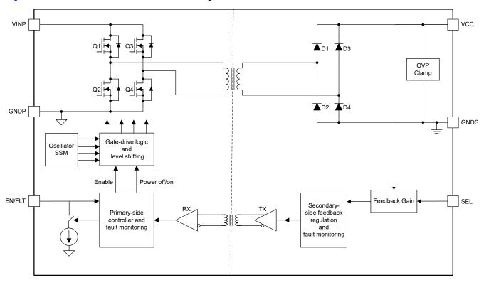
Figure 1-1. Functional Block Diagram
