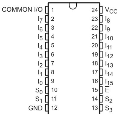
**Figure 4-1. Pin Diagram (SOIC) Package**
