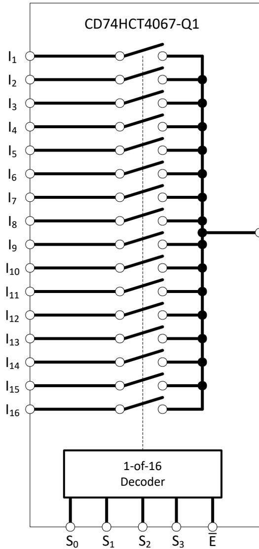
**Figure 1-1. Functional Block Diagram**
