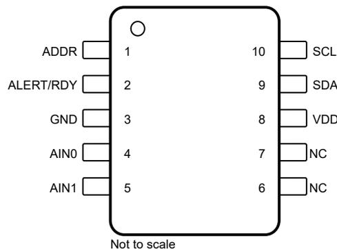
**Figure 4-1. Pin Diagram (VSSOP) Package**
