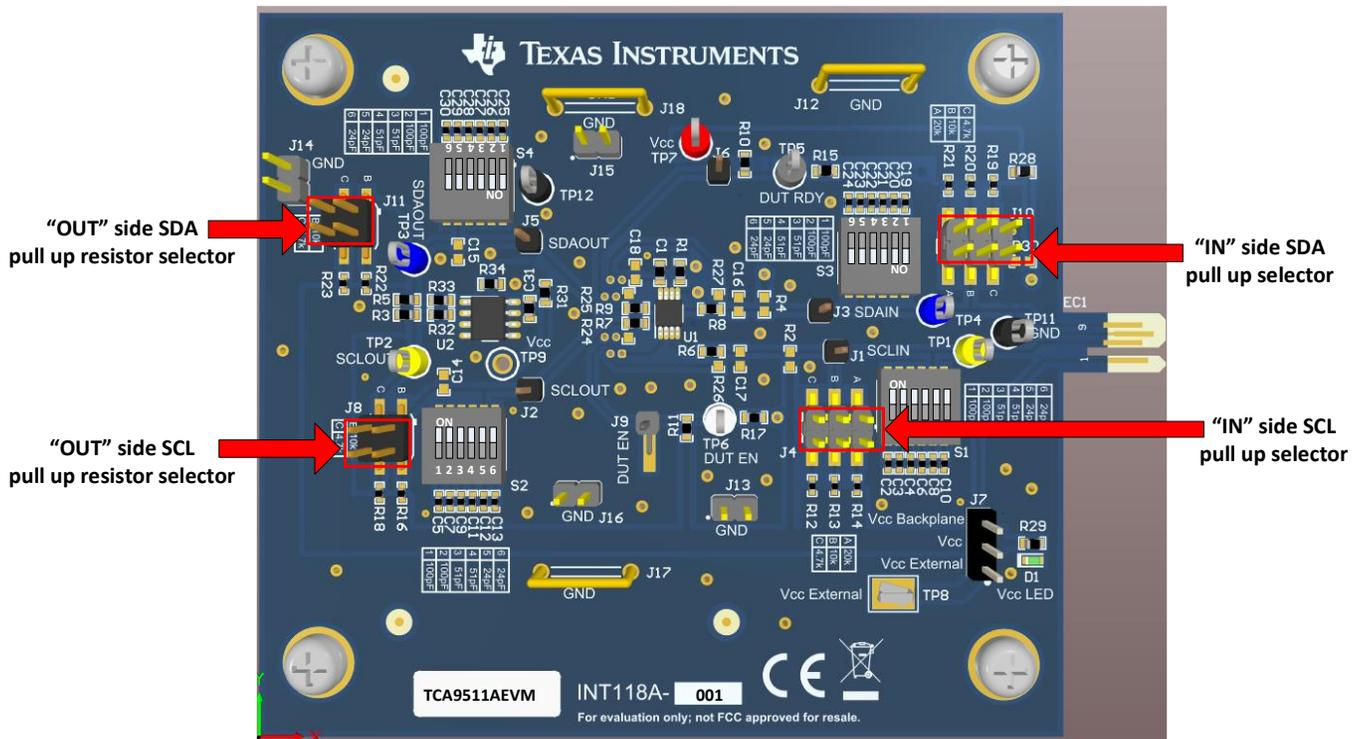
Figure 4. Pull Up Resistor Select
