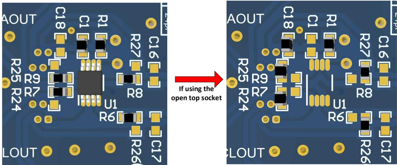
Figure 8. Socket Board set up
