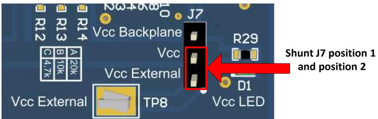
Figure 2.  $V_{CC}$  External Select
