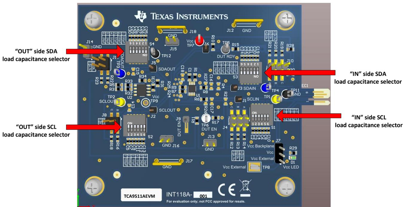
**Figure 5. Load Capacitor Select**
