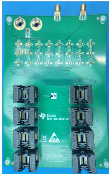
**Figure 3-3. SN54SC6T07-SEP Evaluation Board (Top View)**
