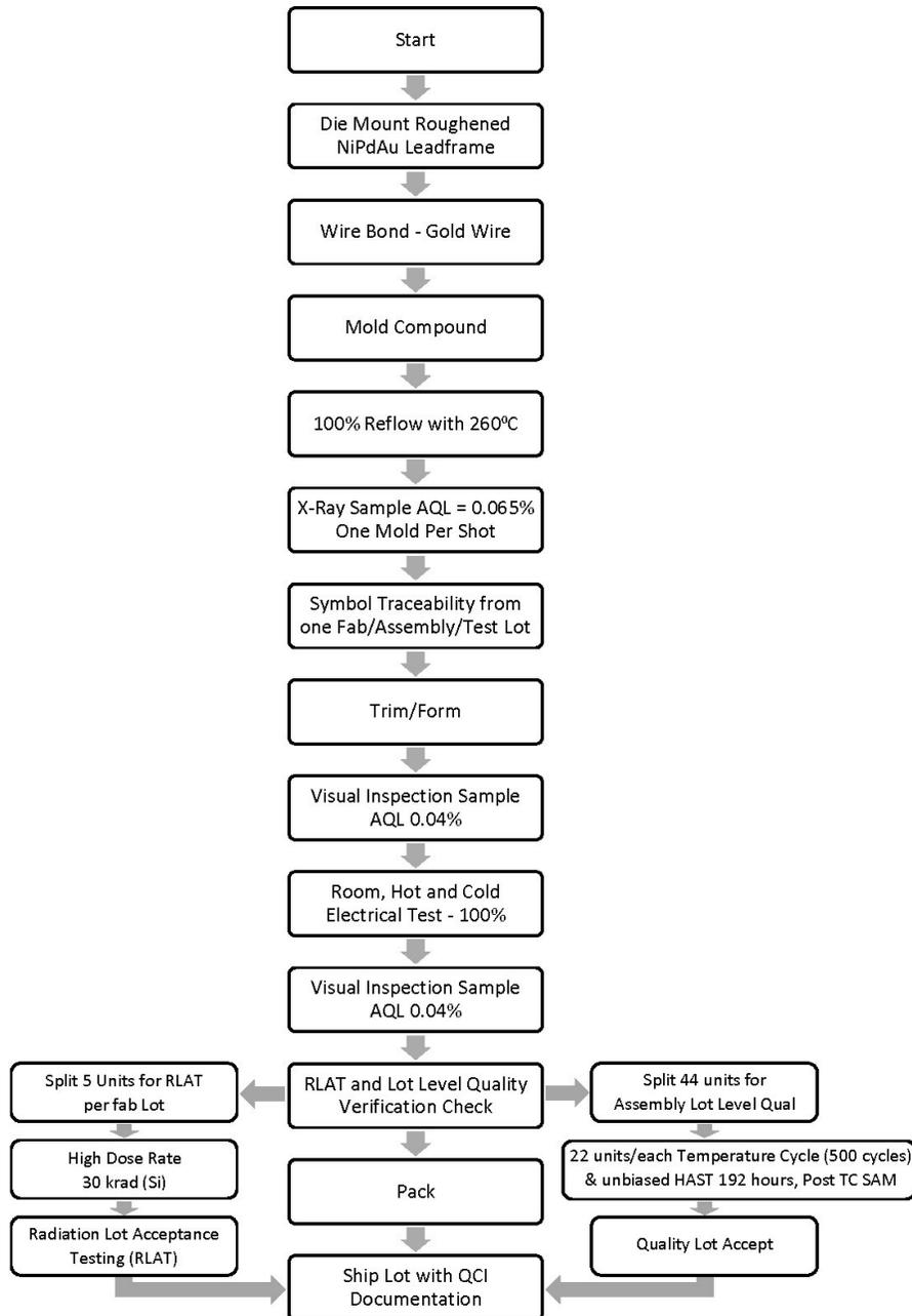
Figure 2-1. SN54SC3T98-SEP Space Enhanced Plastic Production Flow Chart
