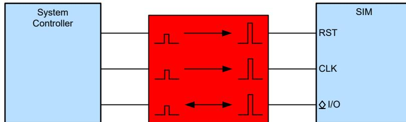
Figure 1. Example SIM Card Voltage Translation Block Diagram
