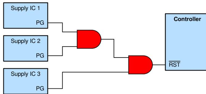
Figure 3-2. Using Logic to Combine Multiple Power-Good Signals
