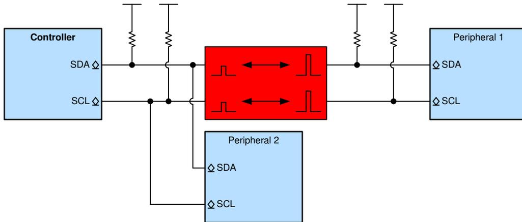
**Figure 3-9. Using Voltage Translation with an I<sup>2</sup>C Communication Bus**
