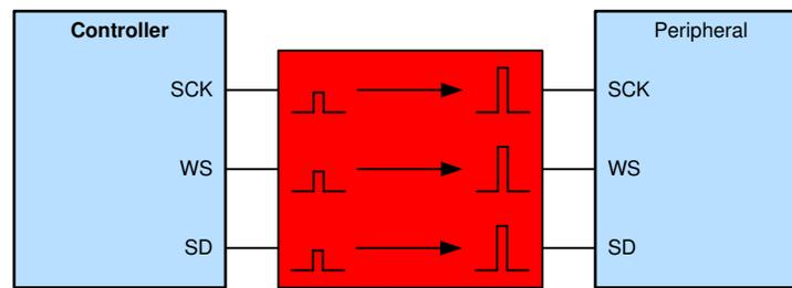
**Figure 3-10. Using Voltage Translation with an I<sup>2</sup>S Communication Bus**
