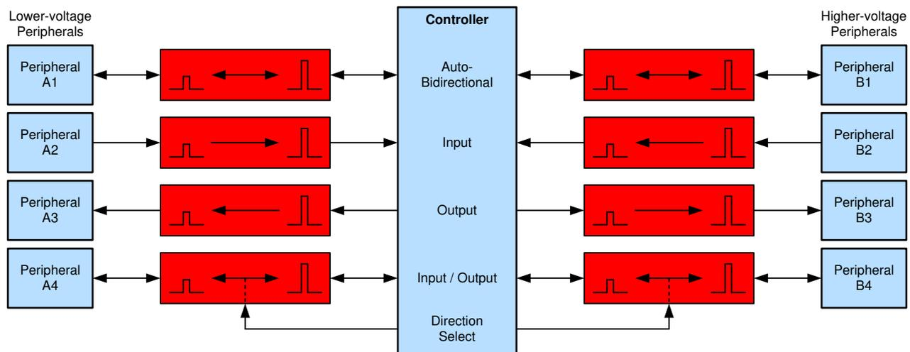
Figure 3-8. Using Voltage Translation with GPIO Communications
