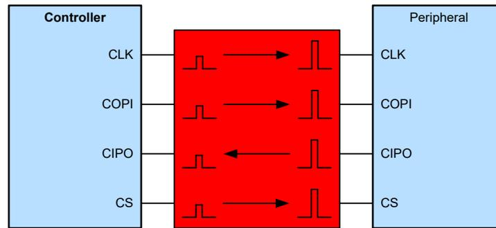
Figure 3-7. Using Voltage Translation with a SPI-Communication Bus
