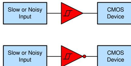
Figure 3-6. Using Schmitt-Trigger Drivers to Remove Noise or Slow Edges from Digital Signals
