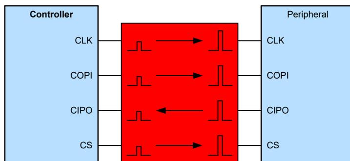
Figure 2-2. Using Voltage Translation with a SPI-Communication Bus
