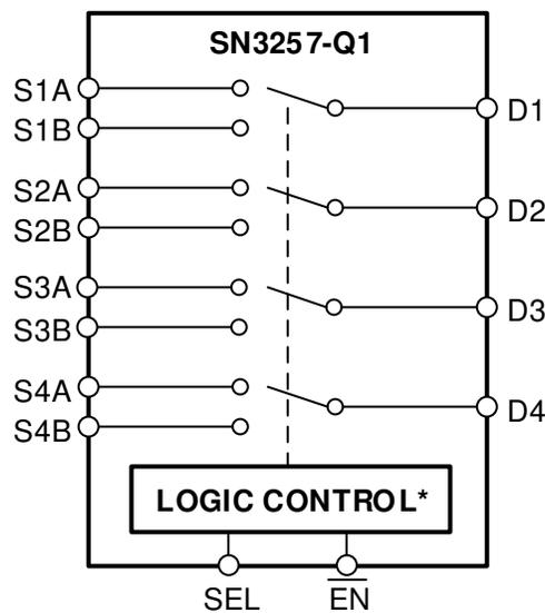
\*Internal 6MΩ Pull-Down on Logic Pins
