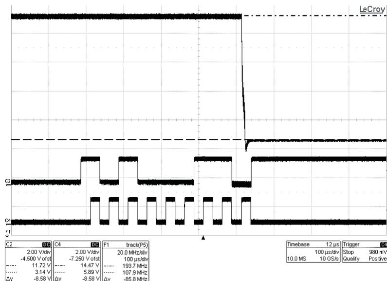
Step 1 to change from 194 MHz to 170 MHz. I2C writeByte a3xh on address 1axh (cr(1axh)=a3xh); the previous contents on that address was a6xh. The change is effective when the last bit on the address 1axh is patterned. C2 is I2C\_SDA, C4 is I2C\_SCK, and F1 is the frequency on Y1.
