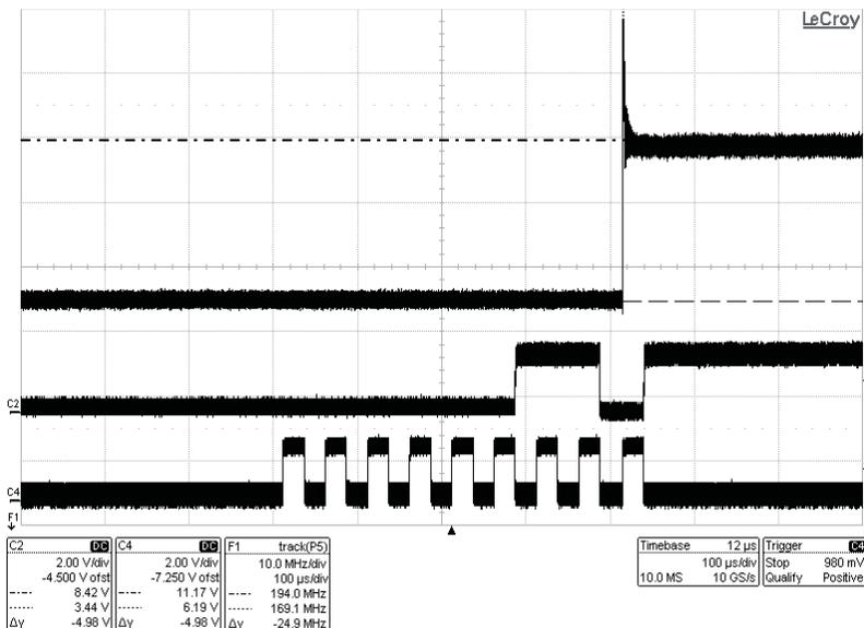
C2 is I2C\_SDA, C4 is I2C\_SCK, and F1 is the frequency on Y1. When byte FS1 (address 13xh) is written to 3xh, PLL1 active setup changes from PLL\_setup0 to PLL\_setup1. In this plot, PLL\_setup0 Y1's frequency is set to 170 MHz, and PLL\_setup1 Y1's frequency is set to 194 MHz.
