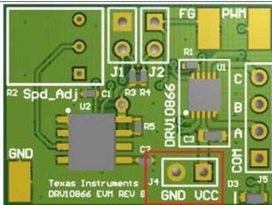
Figure 3. Top View (J4 Power Supply Header)
