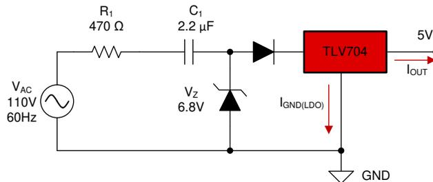
**Figure 2. Basic Capacitive Dropper Circuit With an LDO for 110 V<sub>AC</sub>, 5 V<sub>DC</sub> and 30 mA**
