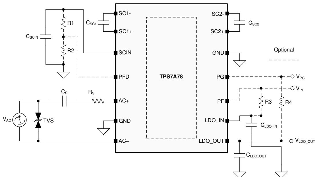
**Figure 3. Typical Cap-Drop Solution Using TPS7A78**
