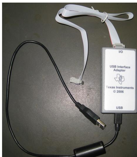
**Figure 3. Picture of USB-TO-GPIO**
