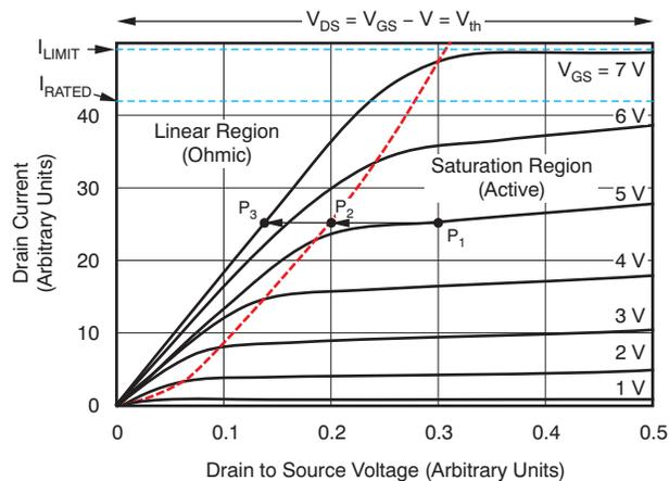
Note: The figure illustrates the relative dependence of the drain-source current,  $I_{DS}$ , on the gate-source voltage,  $V_{GS}$ , and drain-source voltage,  $V_{DS}$ .
