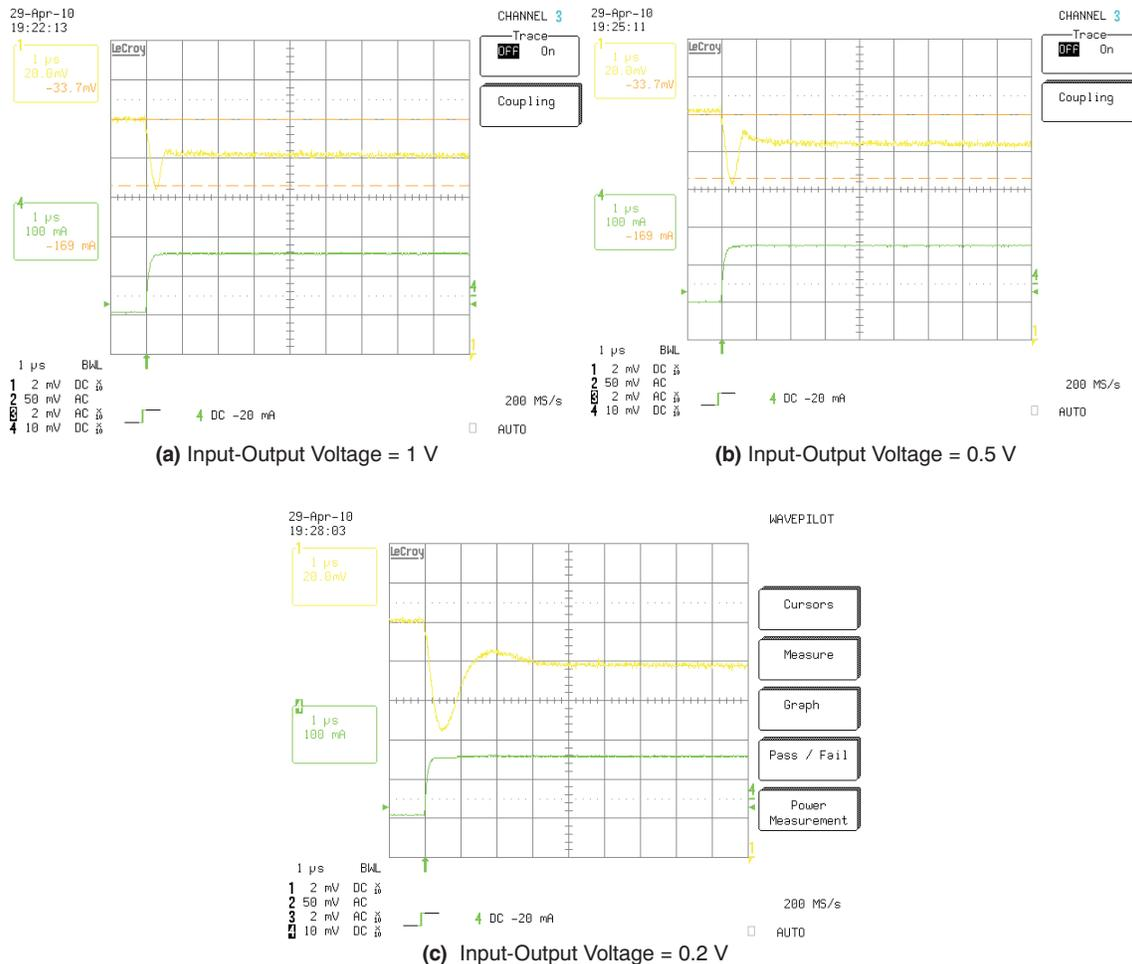
Note: Oscilloscope channel 4 shows the load current step, and channel 1 shows the  $V_{OUT}$  transient response.
