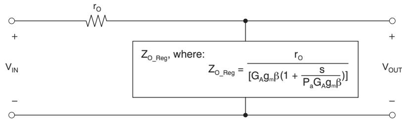
Figure 3. Low-Frequency PSRR Model (Output Impedance Ignored)
