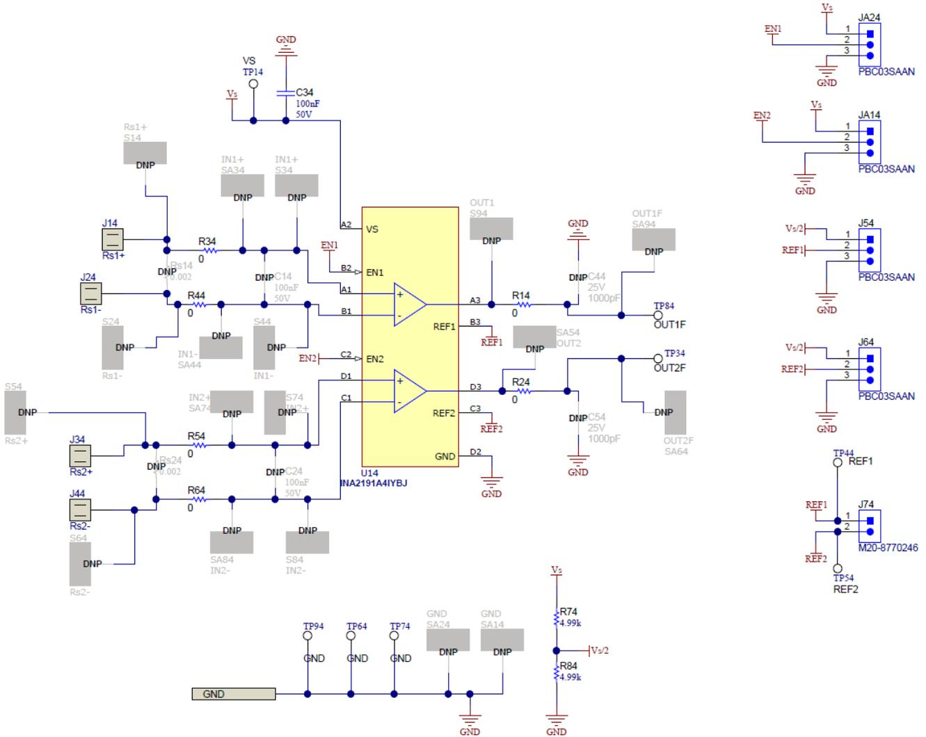
Figure 5-4. INA2191EVM Schematic: Gain A4 Panel
