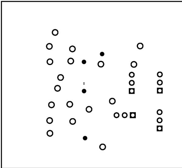
**Figure 5-16. INA2191EVM Bottom Solder for Single Panel**
