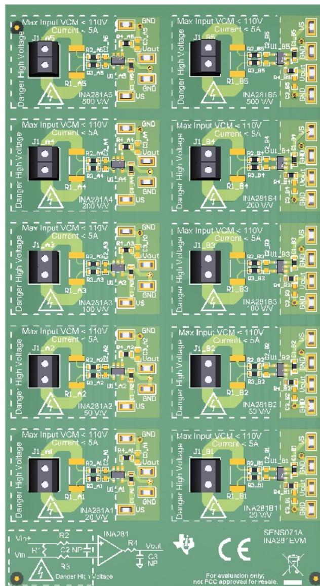
This user's guide describes the characteristics, operation, and use of the INA281 evaluation module (EVM). This EVM is designed to evaluate the performance of the INA281 voltage-output, current shunt monitor in a variety of configurations. Throughout this document, the terms evaluation board, evaluation module, and EVM are synonymous with the INA281EVM. This document also includes a schematic, reference printed-circuit board (PCB) layouts, and a complete bill of materials (BOM).
