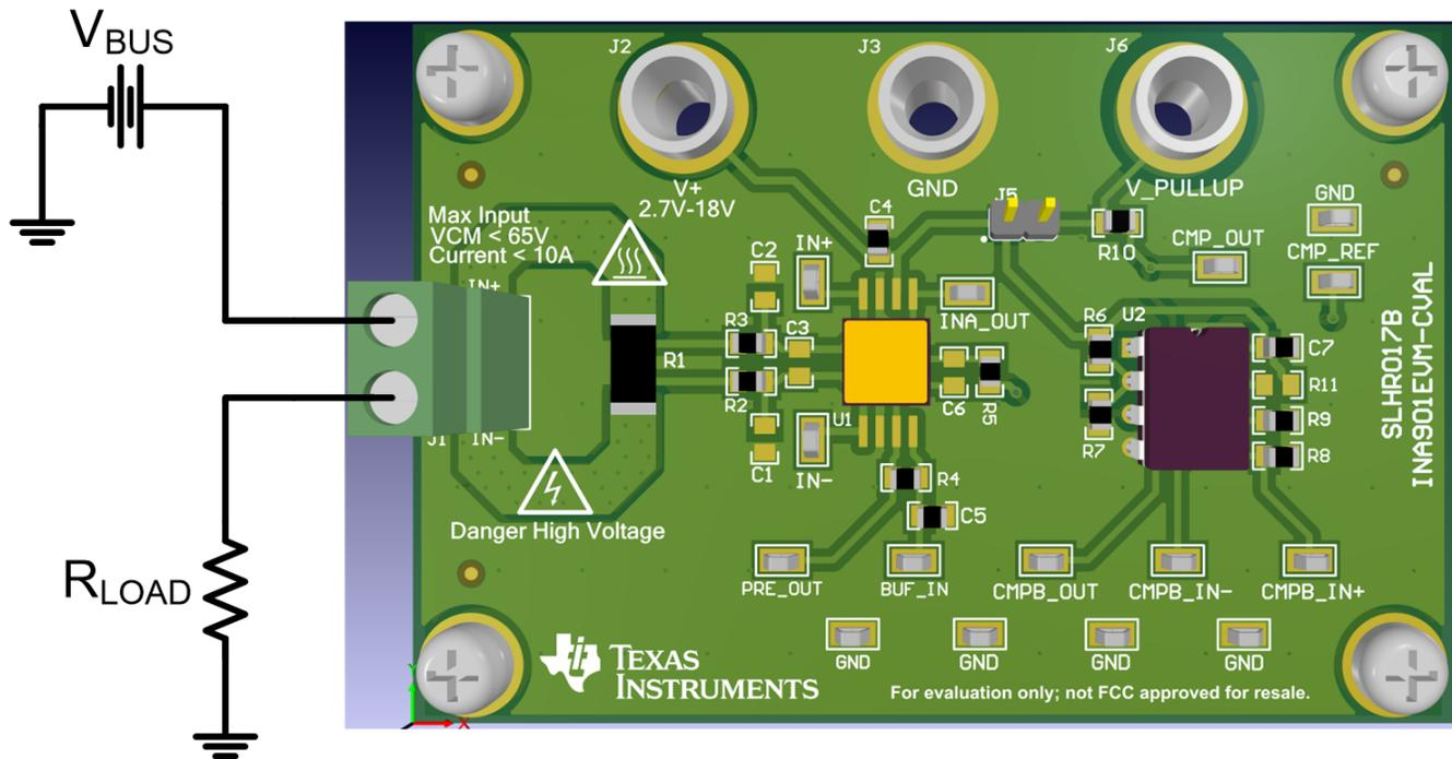
**Figure 1. High-Side Setup Using Onboard Shunt Resistor**
