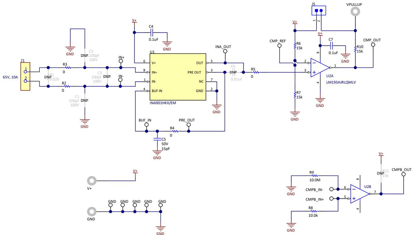
Figure 4. INA901EVM-CVAL Schematic
