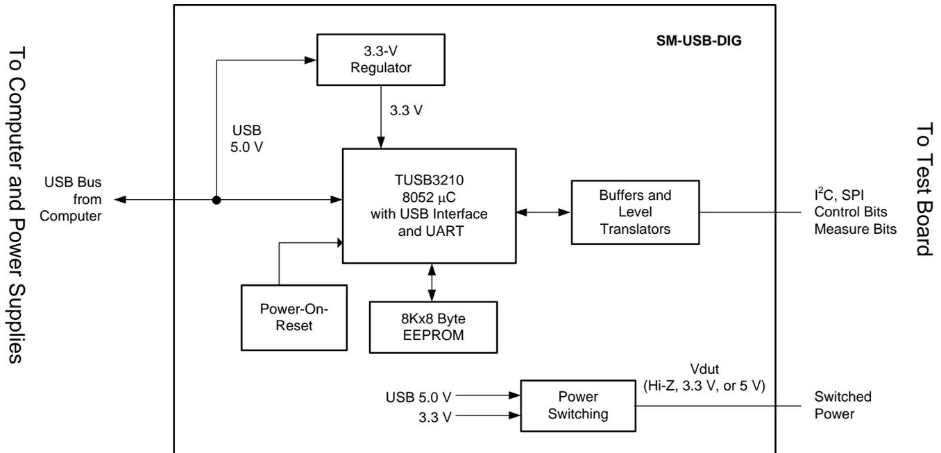
Figure 4. USB DIG Platform Block Diagram
