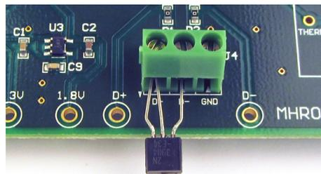
Figure 8. Remote NPN Setup
