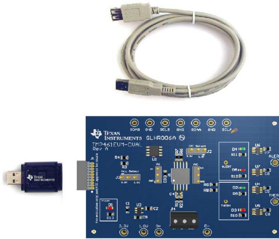
Figure 1. Hardware Included With TMP461EVM-CVAL Kit
