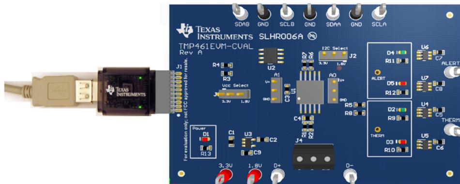
Figure 5. Connecting the SM-USB-DIG Platform
