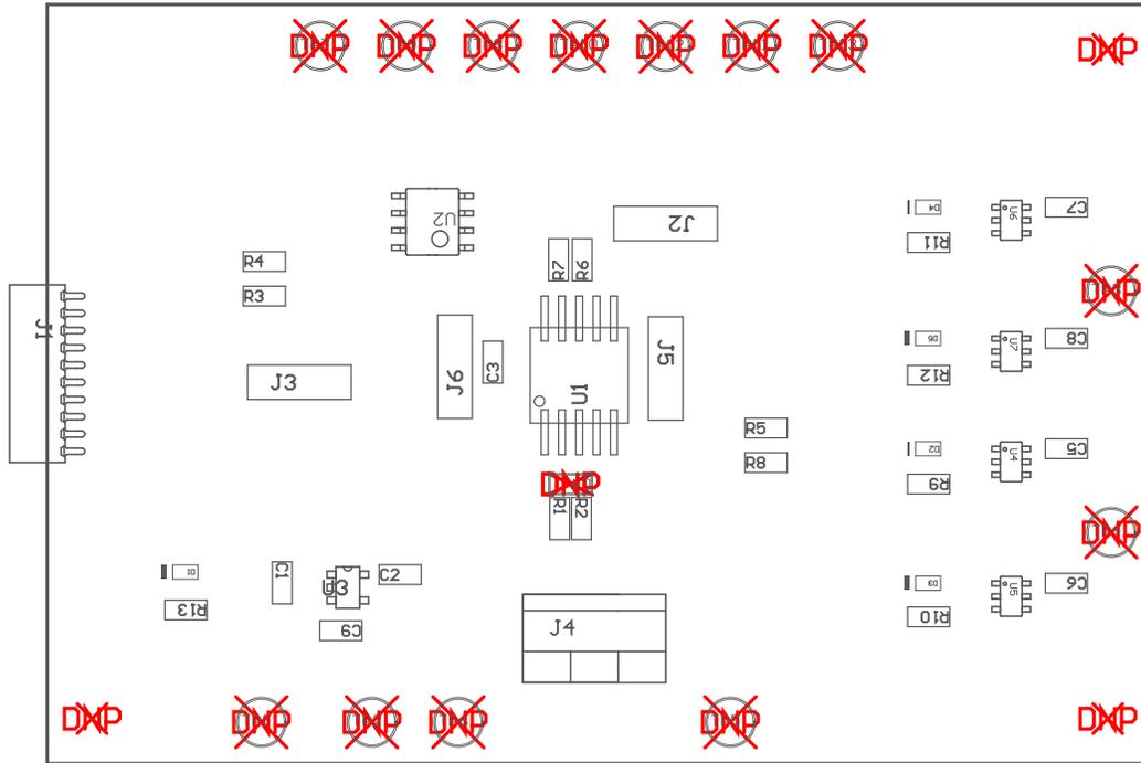
**Figure 21. TMP461EVM-CVAL Components Layout**
