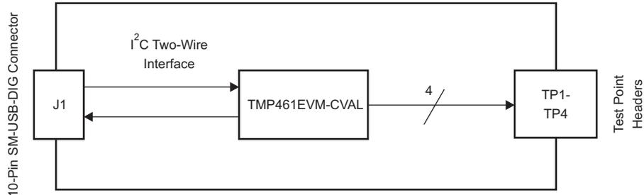
Figure 3. TMP461EVM-CVAL Test Board Block Diagram
