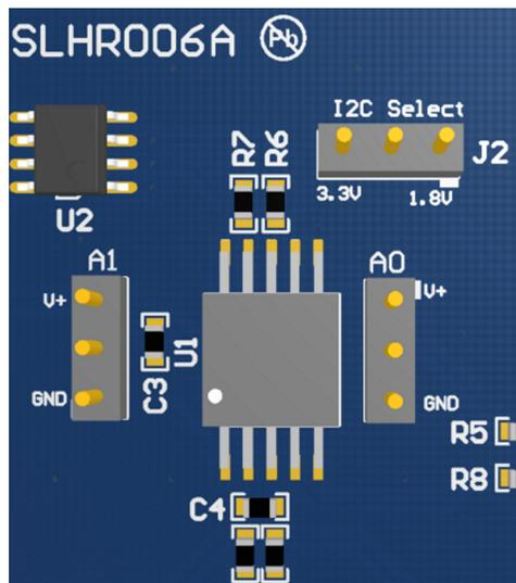
**Figure 9. Slave Address Connections (A0, A1)**
