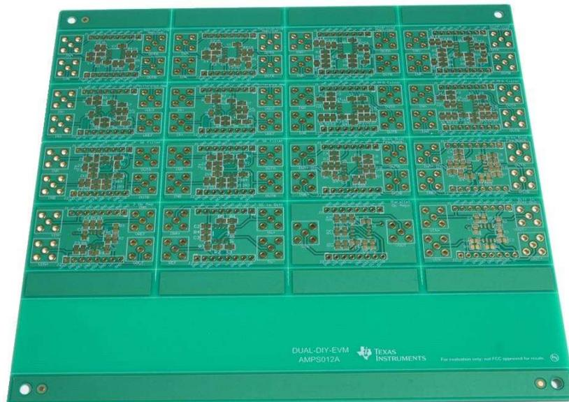
This user's guide contains support documentation for the DUAL-DIYAMP Evaluation Module (EVM). Included is a description of how to set up and configure the EVM, printed circuit board (PCB) layout, schematic, and bill of materials (BOM) of the DUAL-DIYAMP-EVM.
