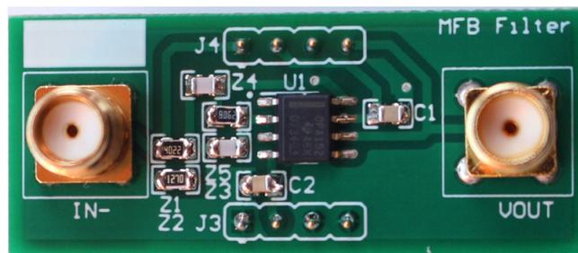
Figure 29. SMA Vertical Connectors
