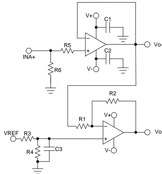
Figure 23. Single-Ended Input to Differential Output Schematic
