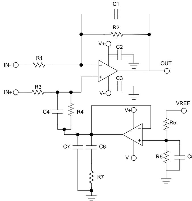
**Figure 13. Difference Amplifier with Reference Buffer Schematic**
