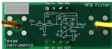
**Figure 31. Wire Connections**
