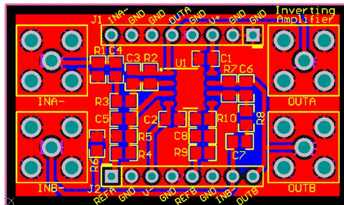
Figure 12. Inverting Amplifier Top Layer PCB Layout
