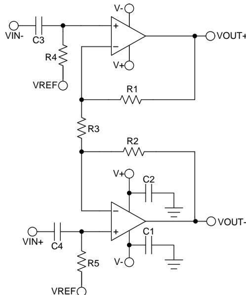
Figure 27. Differential Input to Differential Output Schematic
