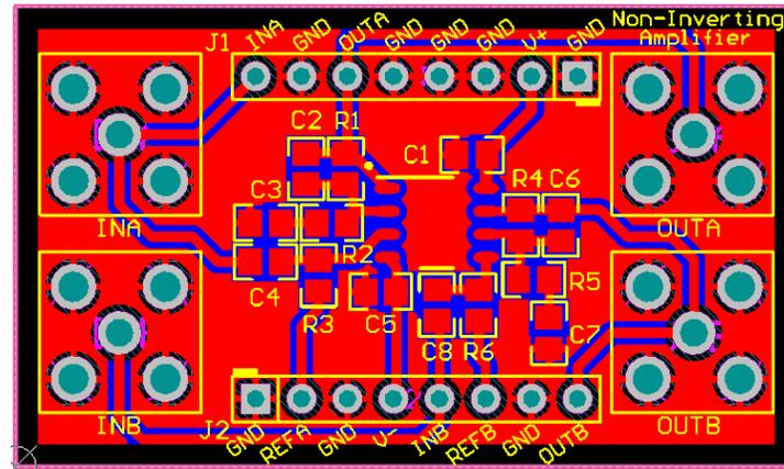
Figure 10. Non-Inverting Amplifier Top Layer PCB Layout
