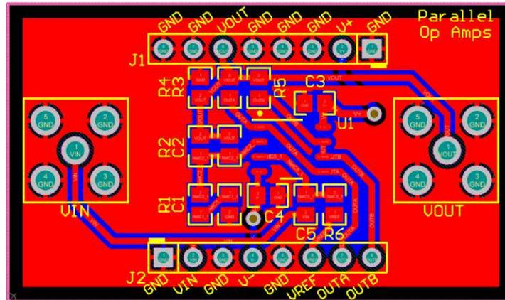
Figure 26. Parallel Op-Amp Top Layer PCB Layout
