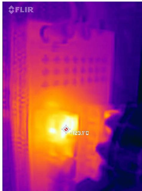
Figure 3-5. SN54SC4T125-SEP Thermal Image for SEL
