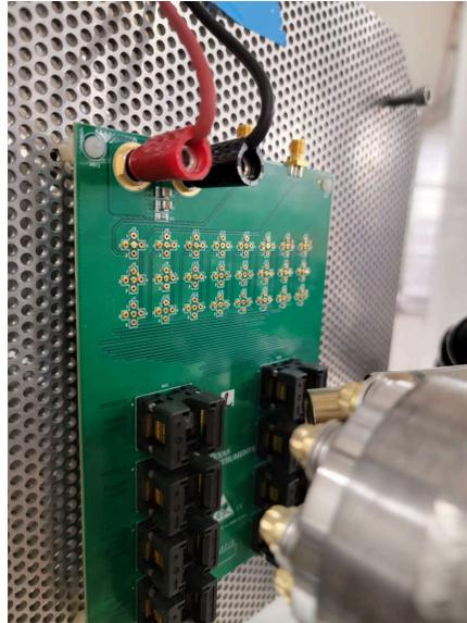
Figure 4-1. SN54SC4T125-SEP Evaluation Board at the MSU FRIB Facility
