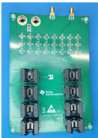
Figure 3-3. SN54SC4T125-SEP Evaluation Board (Top View)
