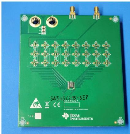
Figure 3-3. SN54SC245-SEP Evaluation Board (Top View)
