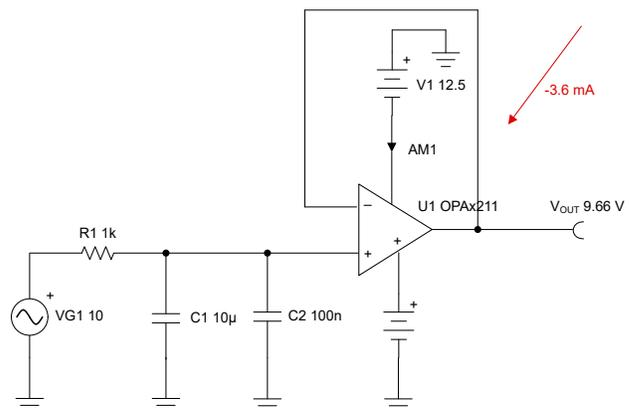
Figure 3. TGC Drive Circuit Using the OPA211
