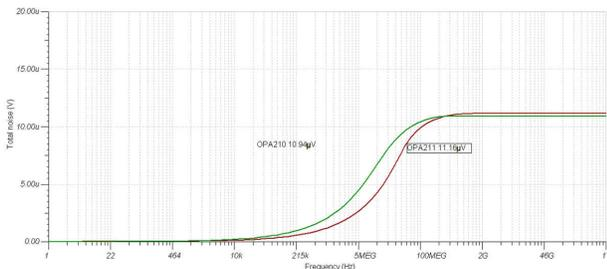
Figure 1. Total Noise of OPA210 and OPA211 in TGC Drive Circuit for Ultrasound
