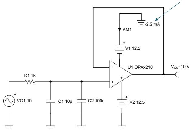
Figure 2. TGC Drive Circuit Using the OPA210
