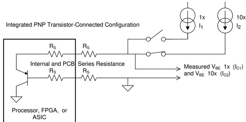
Figure 1-1.  $\Delta V_{BE}$  Measurement with Two Currents
