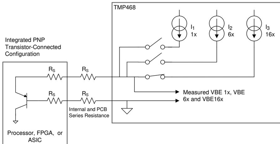
Figure 1-2.  $\Delta V_{BE}$  Measurement with Three Currents
