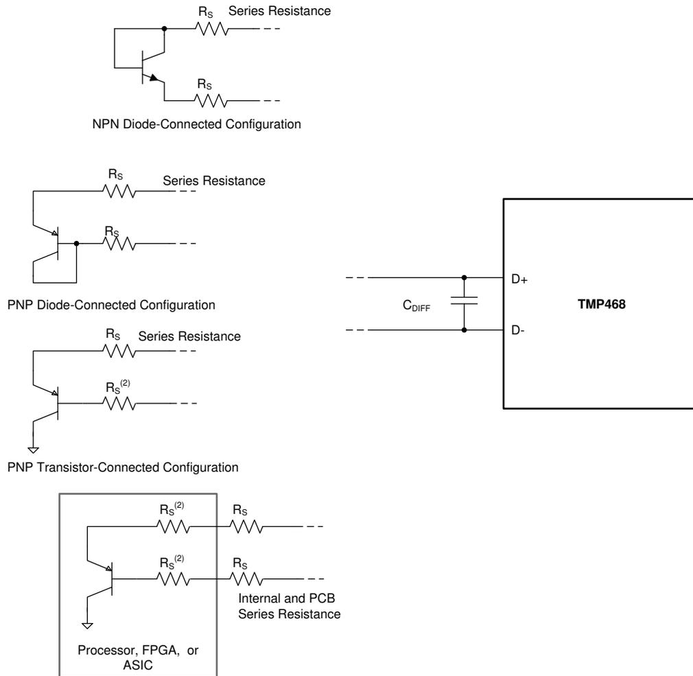
**Figure 3-1. Remote Junction Configurations**
