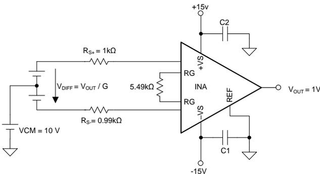
Figure 1. Example Application With  $G = 10$  V/V
