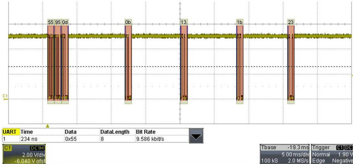
Figure 11. Oscilloscope of 4 Parts Chain Initialization Signal
