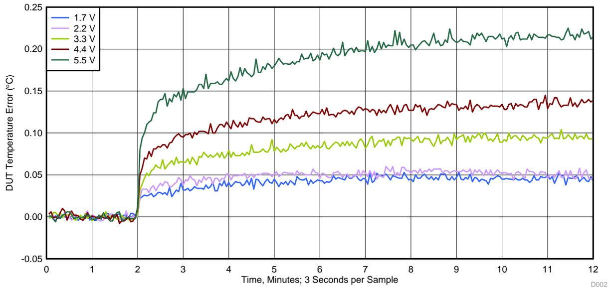
On second minute, TMP107 is switched from one shot mode to continuous 15-ms conversion mode. Data is read back every 3 s.
