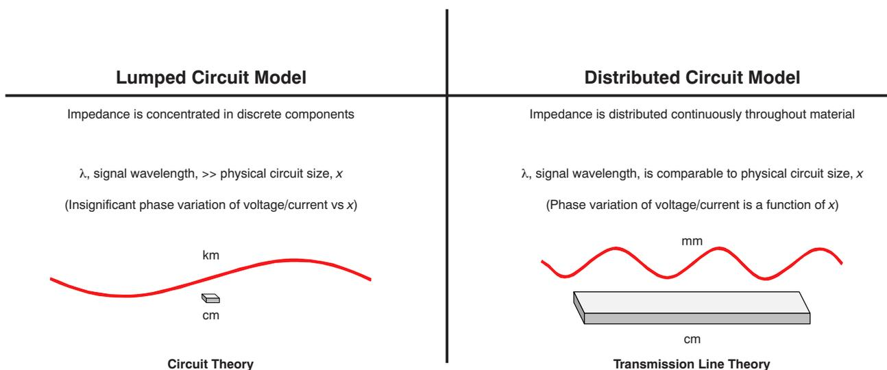
Figure 7. Lumped Circuit Model vs. Distributed Circuit Model
