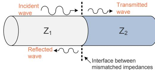
$$\text{Magnitude of reflected voltage wave, } \Gamma = \frac{(Z_2 - Z_1)}{(Z_2 + Z_1)}$$
