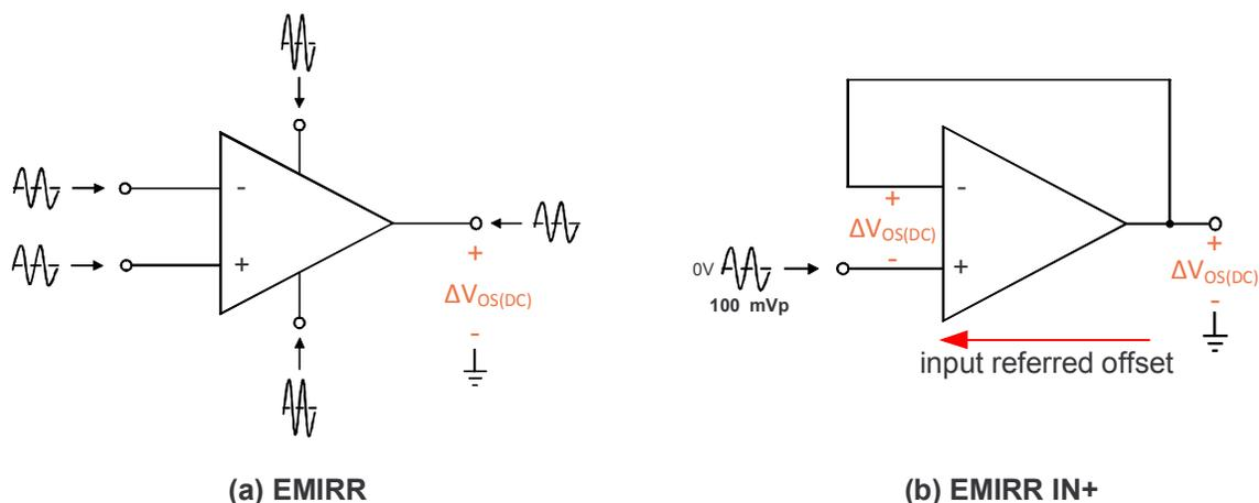
**Figure 5. EMIRR and EMIRR IN+ Measurement Comparison**
