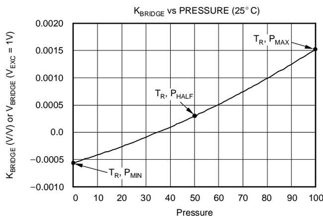
**Figure 2. Output Response of a Bridge Sensor vs Stimulus**
