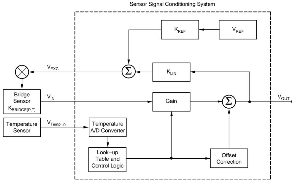
Figure 3. Sensor and Signal Conditioning System
