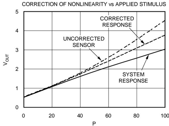
**Figure 4. System Nonlinearity Cancels Sensor Nonlinearity**
