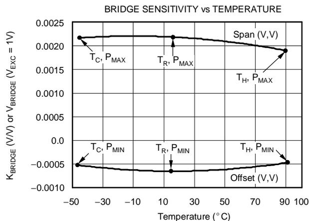
**Figure 1. Output Response of a Bridge Sensor vs Temperature**
