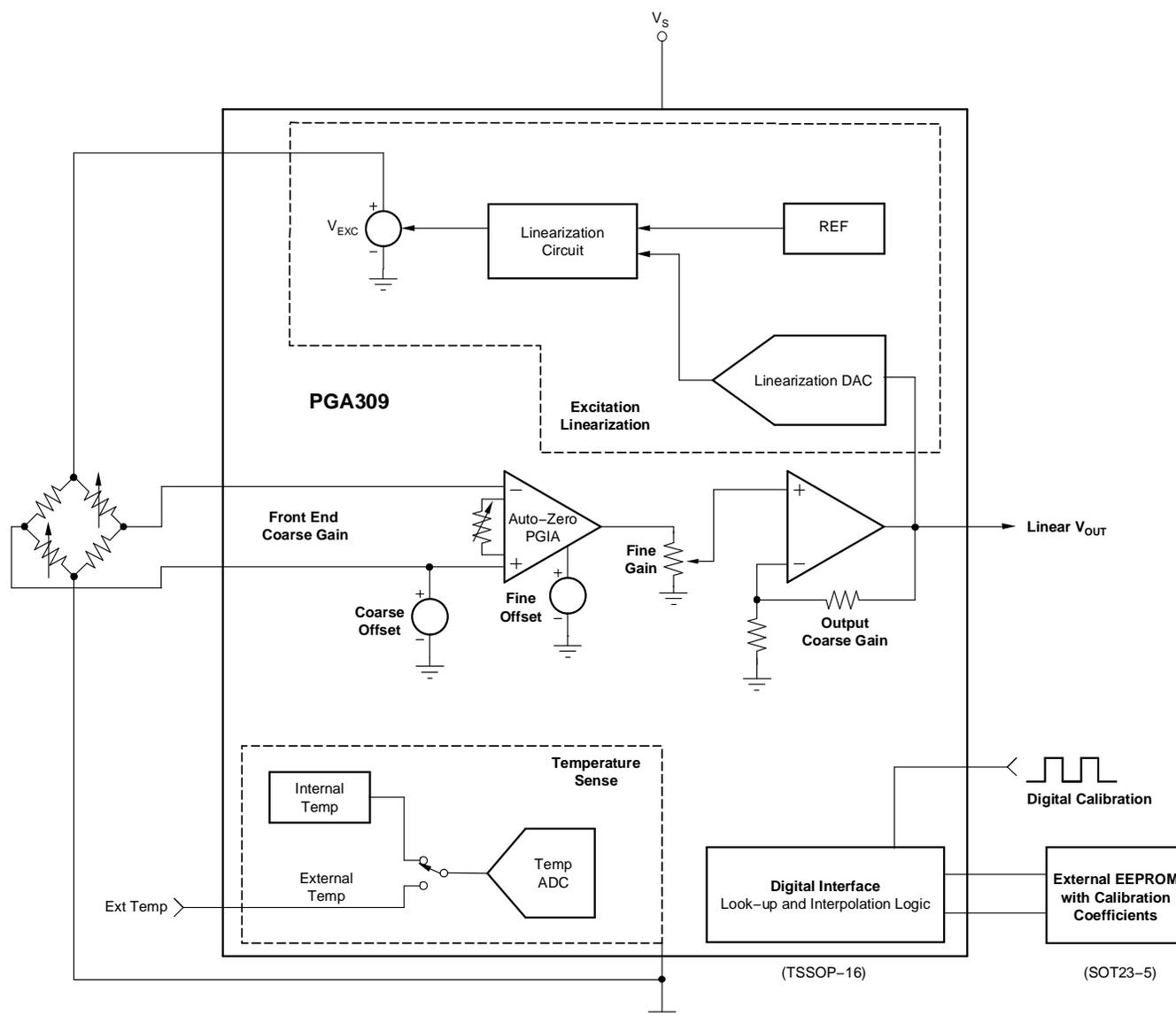
**Figure 8. Block Diagram of PGA309 Integrate Sensor Signal Conditioning System**
