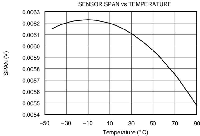
Figure 5. Sensor Span Drift
