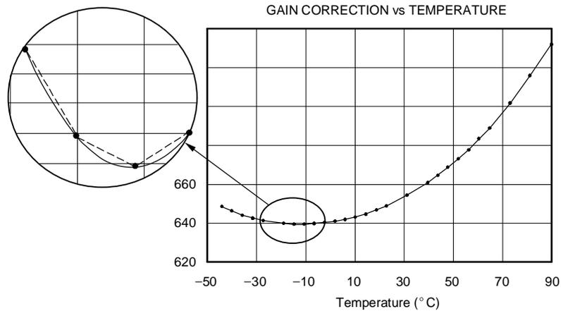
Figure 7. Error Caused by Interpolation
