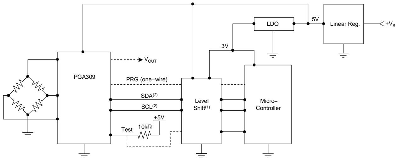
Notes: (1) May be one resistor and internal port pin ESD diode.
