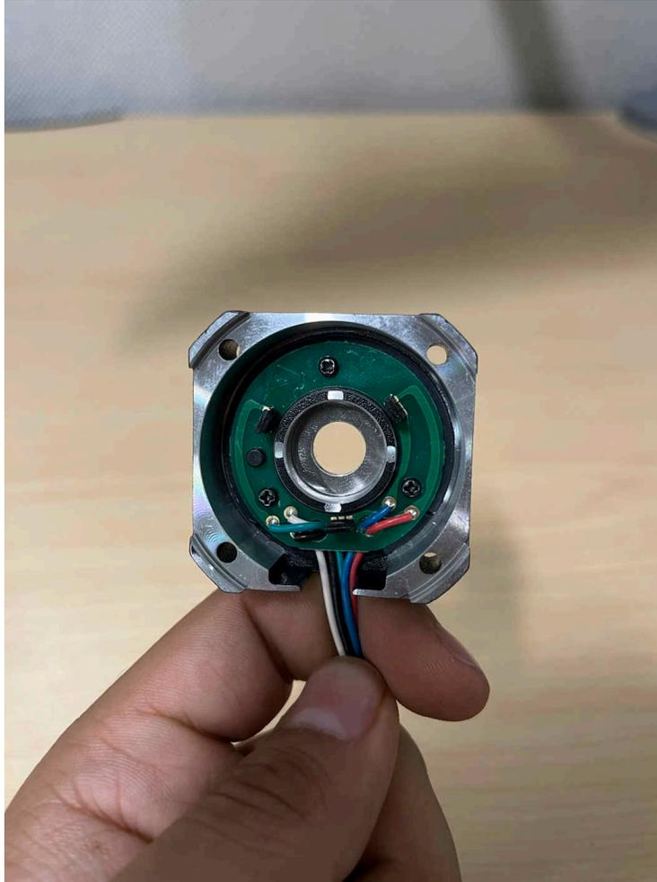
**Figure 3-5. Hall Sensor Board Removal**
