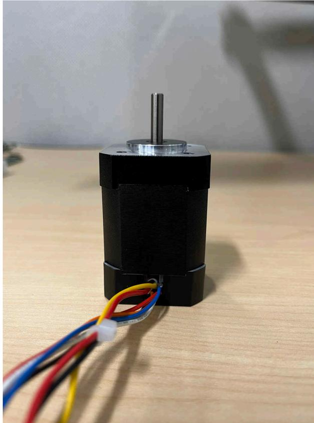
**Figure 3-7. BLDC Motor Connections**
