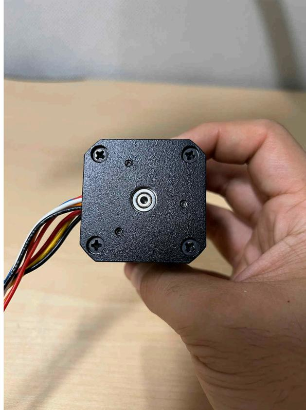
**Figure 3-4. BLDC Motor (Bottom)**
