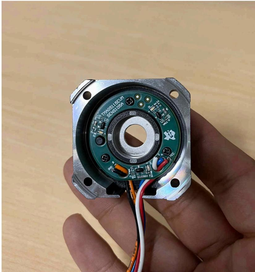
**Figure 3-6. TMAG5115EVM on NEMA17 Motor Module**
