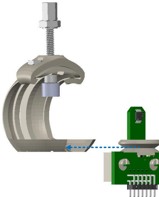
**Figure 2-11. Clip Base Connection to Orbital Arm**
