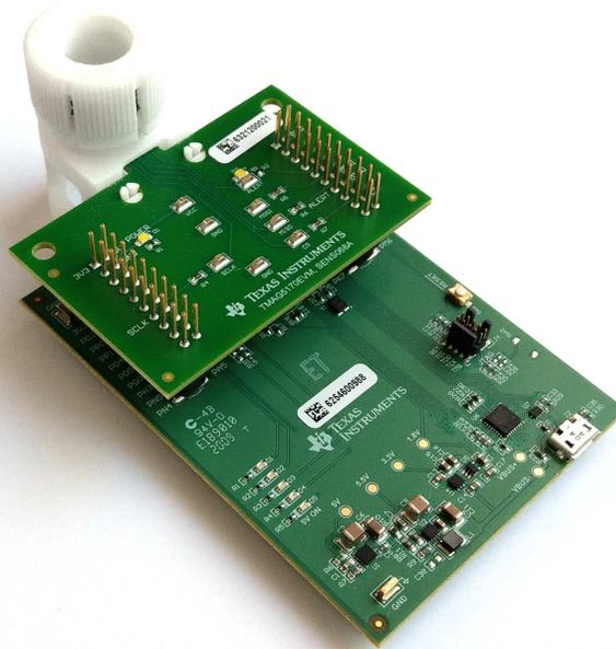
**Figure 9. Rotate & Push Module on EVM**
