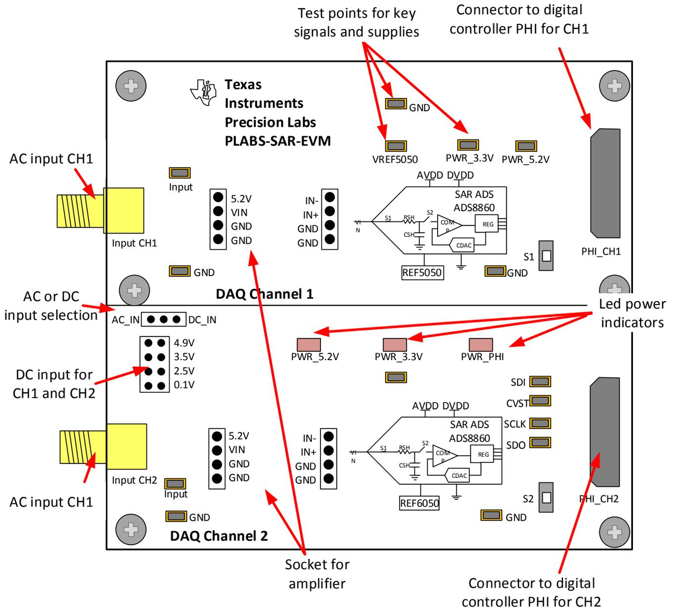
Figure 2. Overview of Features on CH1 and CH2
