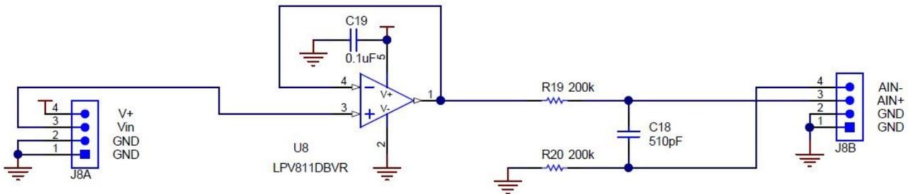
Figure 47. LPV811 Nanopower
