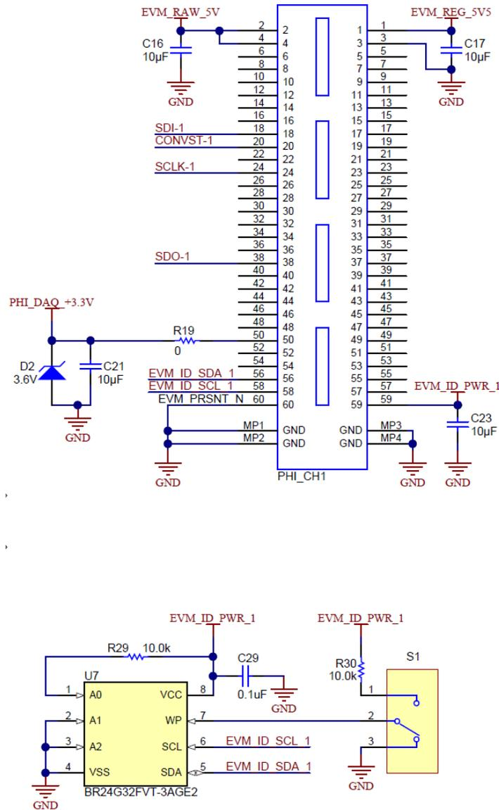
Figure 8. Connection to the PHI Controller and EEPROM
