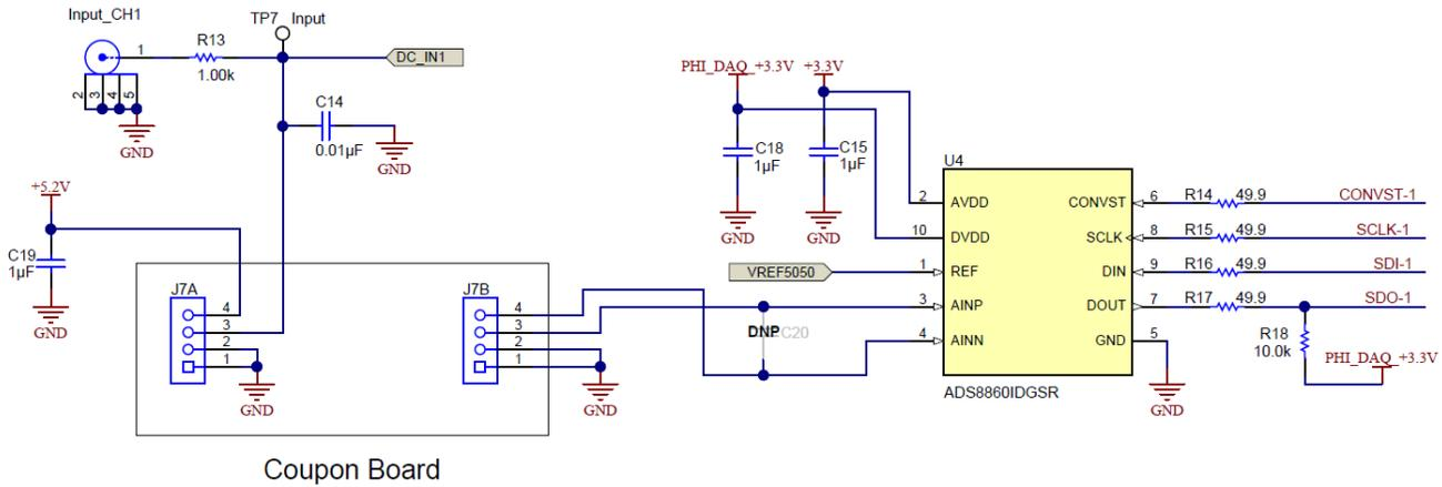
Figure 3. Amplifier and ADC Input (CH1 and CH2)
