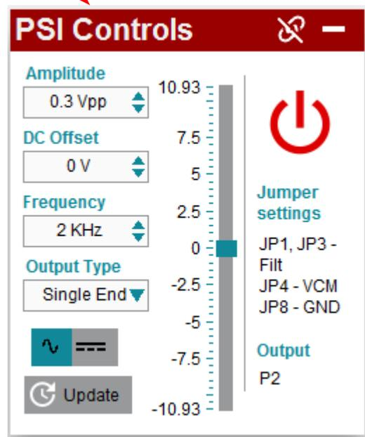
Below the jumper settings are the correct jumper connections for proper operation
