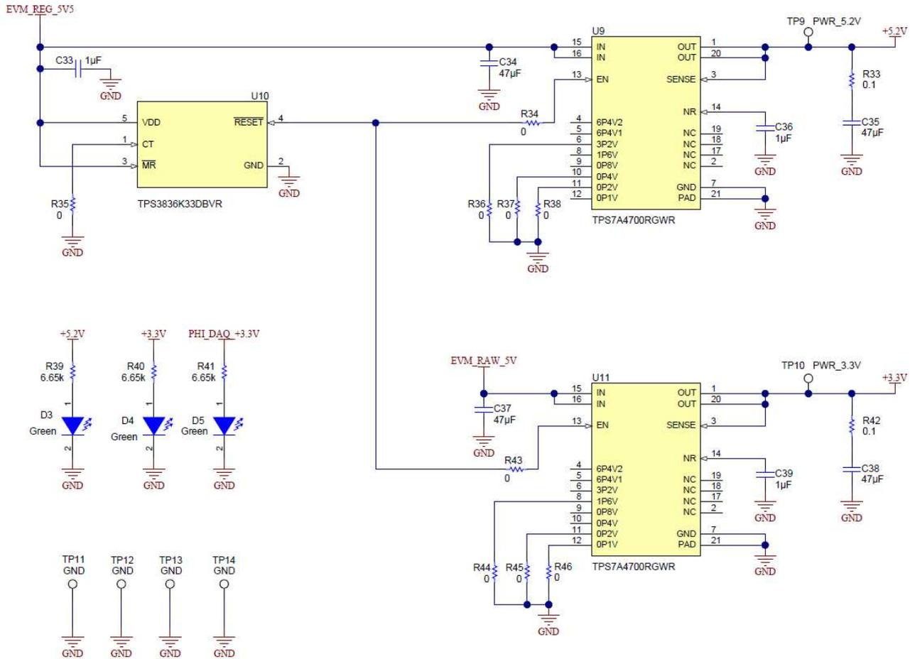
Figure 7. Power Subsection (CH1 and CH2)
